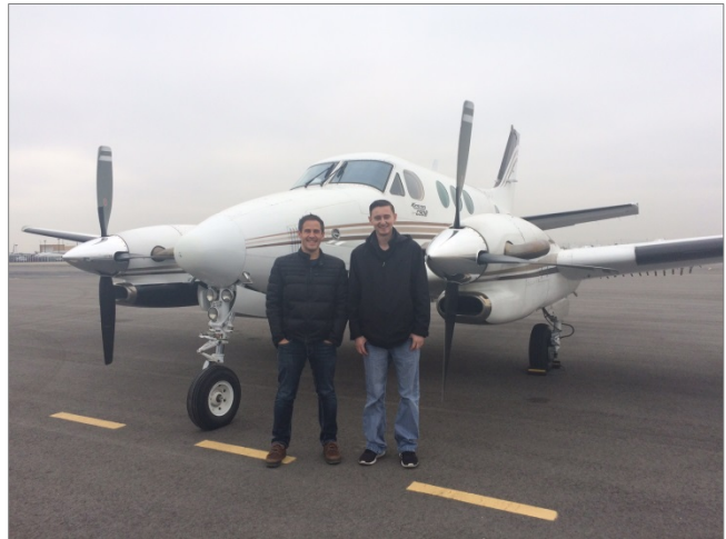
Figure 6. A WMI King Air C90 is pictured, with flight crew, on another current winter orographic seeding program in the Rocky Mountains of the Northern U.S. The burn-in-place flares can be readily seen behind the wing (right). WMI photograph by Brook Mueller.
