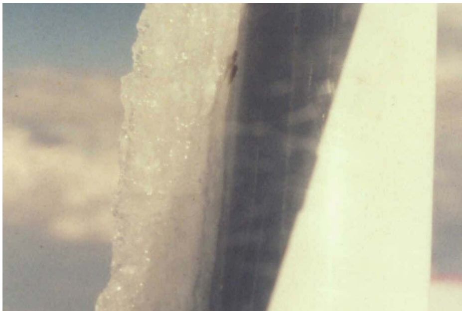
Figure 2.2 - A rime strut on the airframe of University of Wyoming cloud physics Beechcraft Queen Air N10UW. The ice buildup occurred on two consecutive passes through the Elk Mountain cap cloud, and was estimated to be about 1.5 to 2.0 inches thick. (The dark band across the center is shadow.) An immediate full-power descent was required to land the aircraft safely back in Laramie. (Photograph courtesy of B. Boe.)
