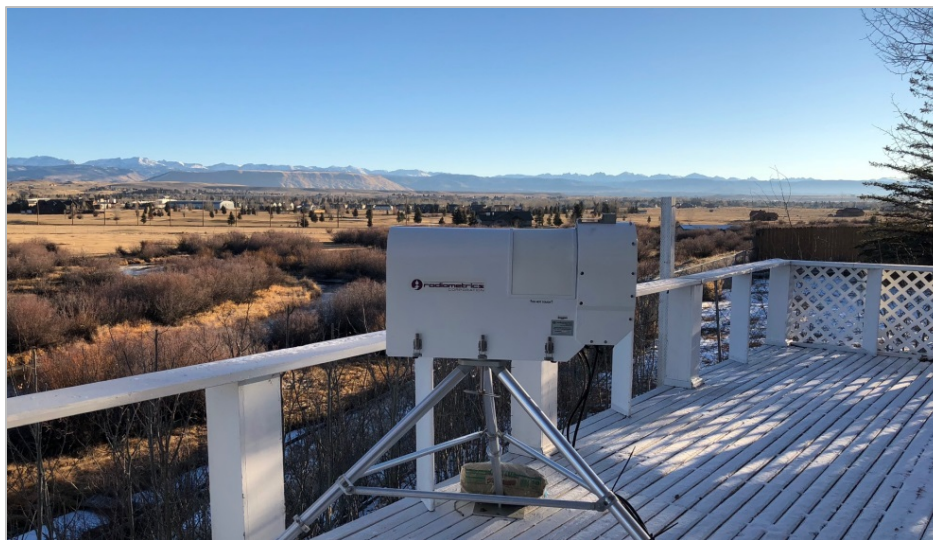
Figure 11. The radiometer is shown here, at the residence of the project meteorologist, near Pinedale. The instrument observes in the direction perpendicular to its axis, so as aligned here, it is configured to take measurements over the Wind River Range in the distance. As utilized in 2018-2019, however, it was zenith-pointing. (WMI photograph by Dan Gilbert.)
