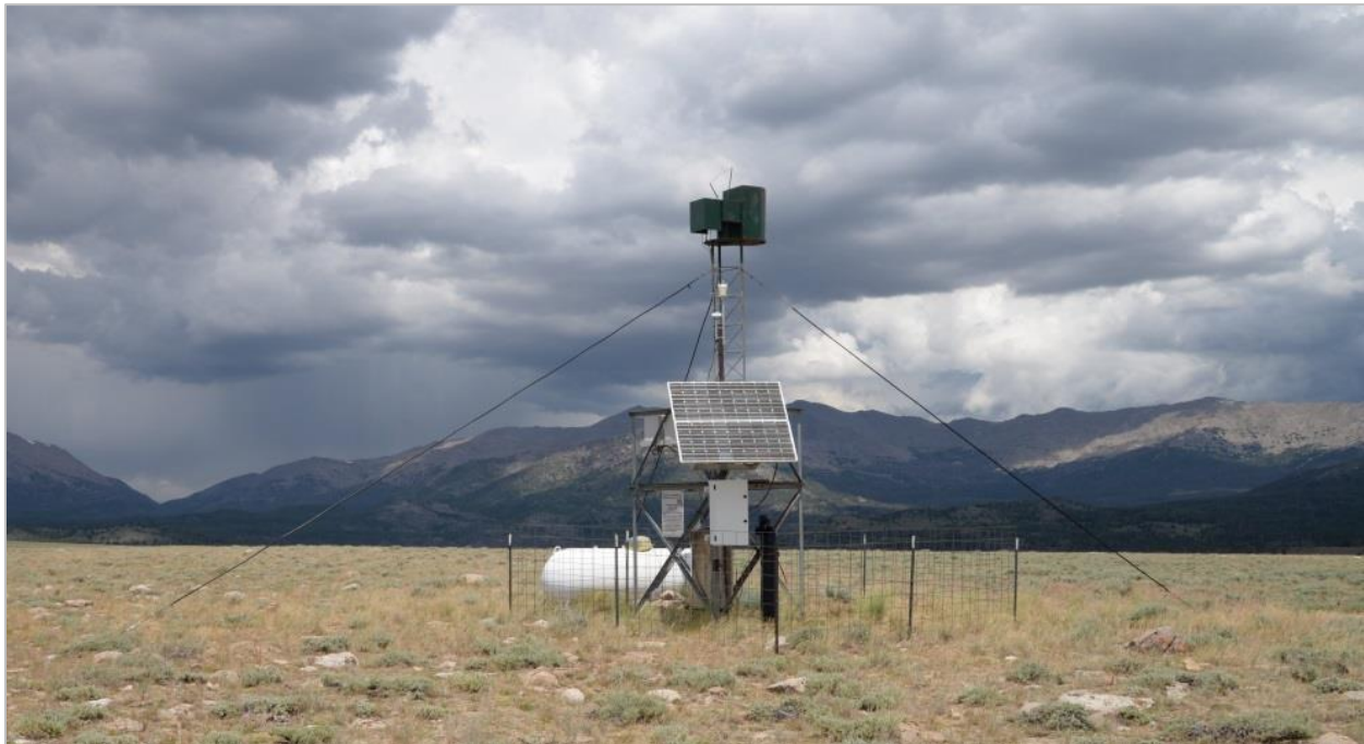
Figure 1. The ice nucleus generator sited at White Acorn Ranch on the west flank of the Wind River Range (WMI photograph). For the locations of all the generators, see Figure 5.
