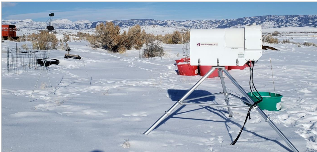
Figure 14. The radiometer is shown here, at the East Fork generator site near Boulder, WY. The instrument observes in the direction perpendicular to its axis, so as aligned here, it is configured to take measurements over the Wind River Range in the distance. The East Fork ice nucleus generator can be seen in the background, left. Photo by WMI Meteorologist Adam Brainard.
