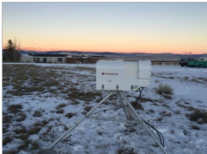
Figure 4 (right). The radiometer sited near Cora, WY. The instrument does not transmit, but passively measures the atmospheric liquid water and water vapor. (WMI photograph by Daniel Gilbert)
