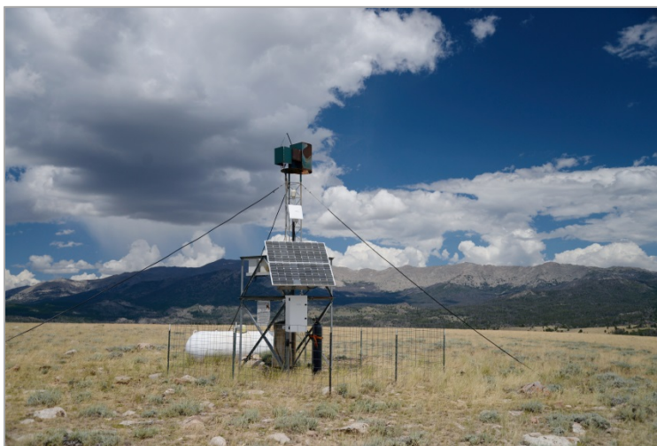
Figure 1 (right). The ice nucleus generator sited at White Acorn Ranch on the southwest flank of the Wind River Range (Weather Modification Inc., photograph). For the locations of all the generators, see Figure 2.
