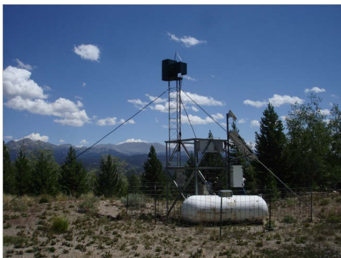
Figure 1. The ice nucleus generator sited at Big Sandy Opening on the southwest flank of the Wind River Range (WMI photograph). For the locations of all the generators, see Figure 2.
