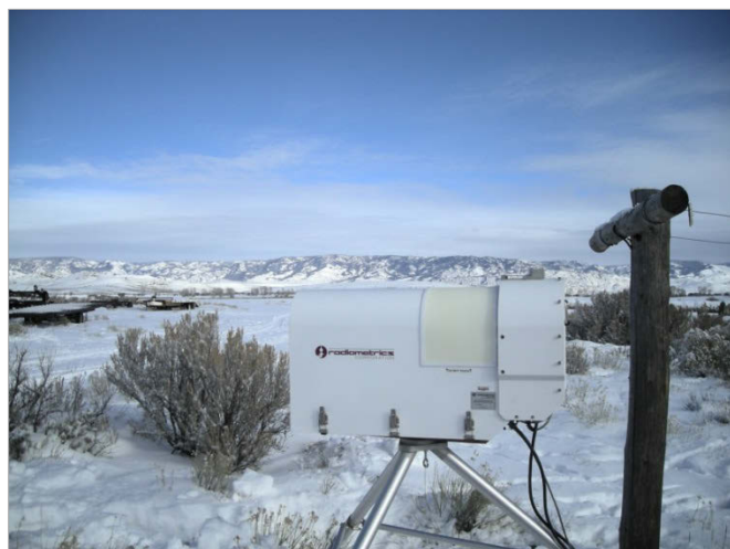
Figure 4. The radiometer sited near Boulder, WY. The instrument does not transmit, but passively measures the atmospheric liquid water and water vapor. (NCAR photograph by Daniel Breed.)
