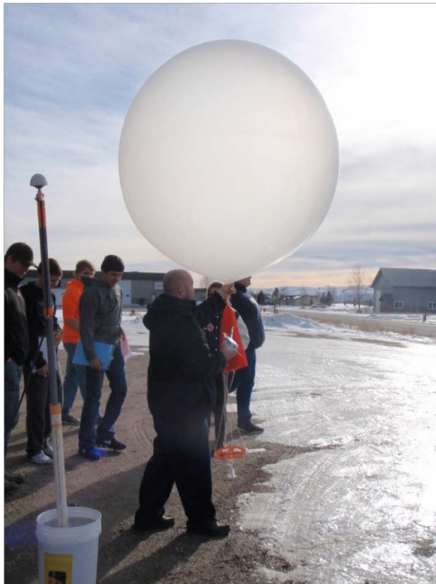
Figure 5. Pinedale high school students and staff learn how to release weather balloons at the WMI shop during a 2014-2015 public outreach event. Sounding data were provided for further examination in class. The instrumentation is contained in the little white package being held in the right hand, while the balloon is held in the left (SCCD photograph by Kathy Raper).
