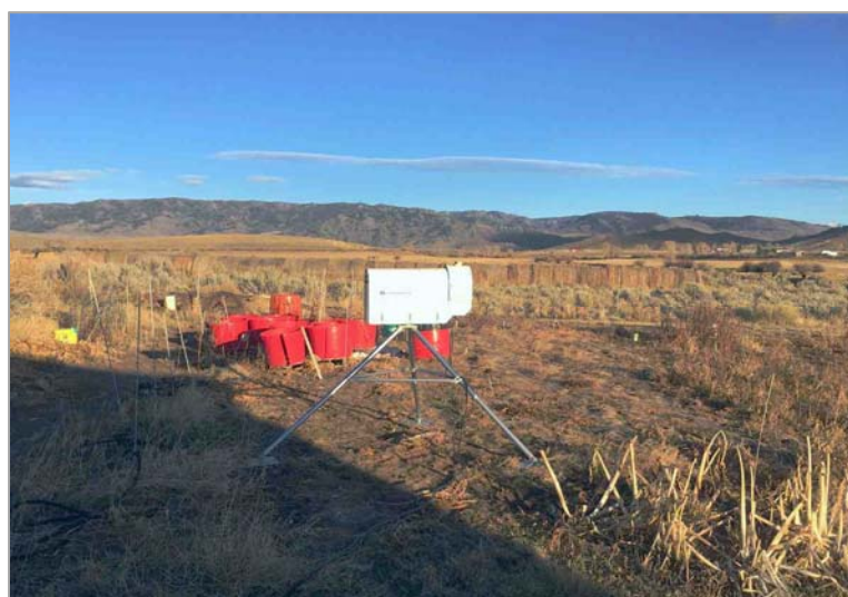
Figure 11. The radiometer sited near Boulder, WY. The instrument does not transmit, but passively measures the atmospheric liquid water and water vapor. (WMI photograph by Daniel Gilbert.)
