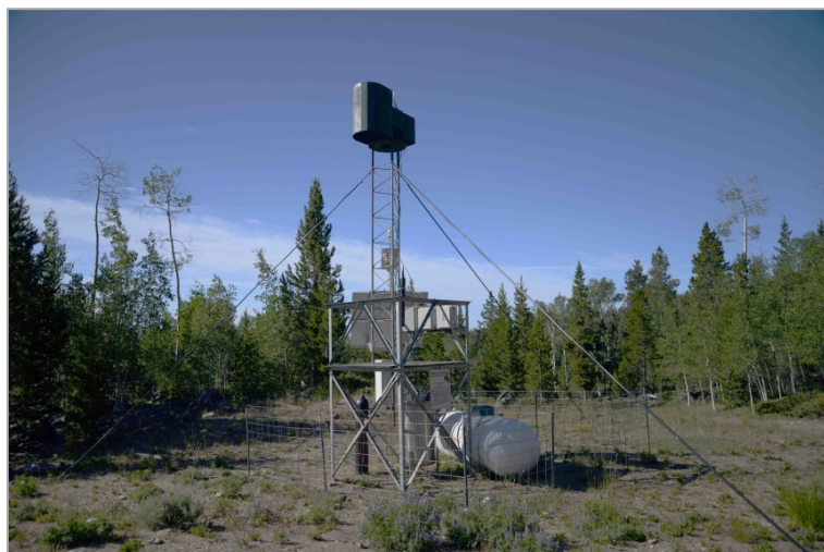
Figure 1. The ice nucleus generator sited at Big Sandy Opening on the southwest flank of the Wind River Range (WMI photograph). For the locations of all the generators, see Figure 5.
