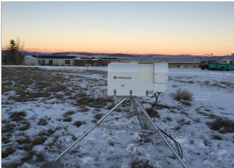
Figure 10. The radiometer sited near Cora, WY. The instrument does not transmit, but passively measures the atmospheric liquid water and water vapor. (WMI photograph by Daniel Gilbert)
