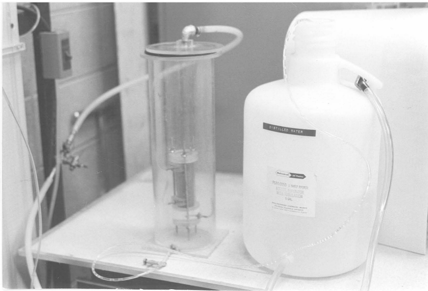
Figure 7. Apparatus for saturating sample for K(h) test.
