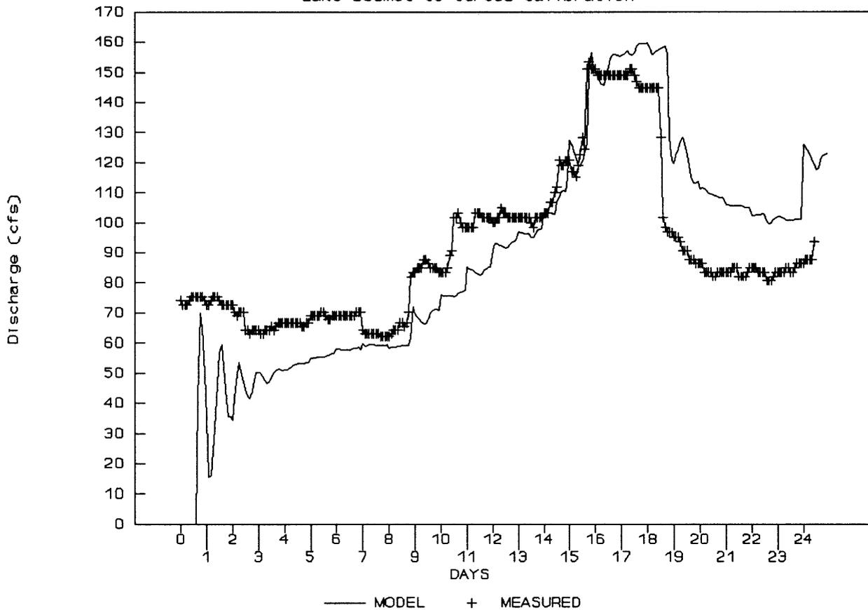
Figure 6. Piney Creek 1984 Reservoir Release, Lake Desmet to Ucross Model Calibration
