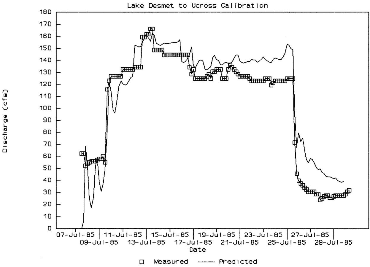
Figure 12. Piney Creek 1985 Reservoir Release, Lake Desmet to Ucross Model Calibration.
