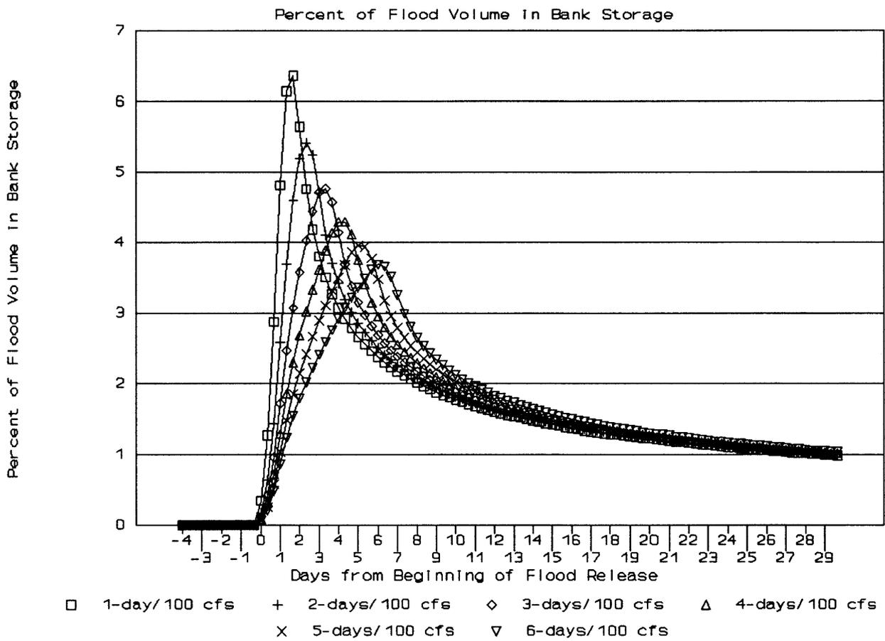
Figure 23. Green River Modeling Results, Percent of Flood Volume in Bank Storage with Varying Duration of Reservoir Release.
