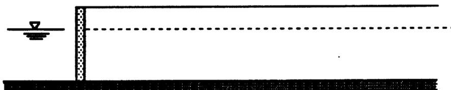
Semi-infinite aquifer with a permeable confining bed separating the stream and the aquifer.
