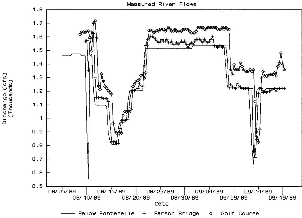
Figure 16. Green River 1989 Reservoir Release, Measured River Flow Hydrographs.
