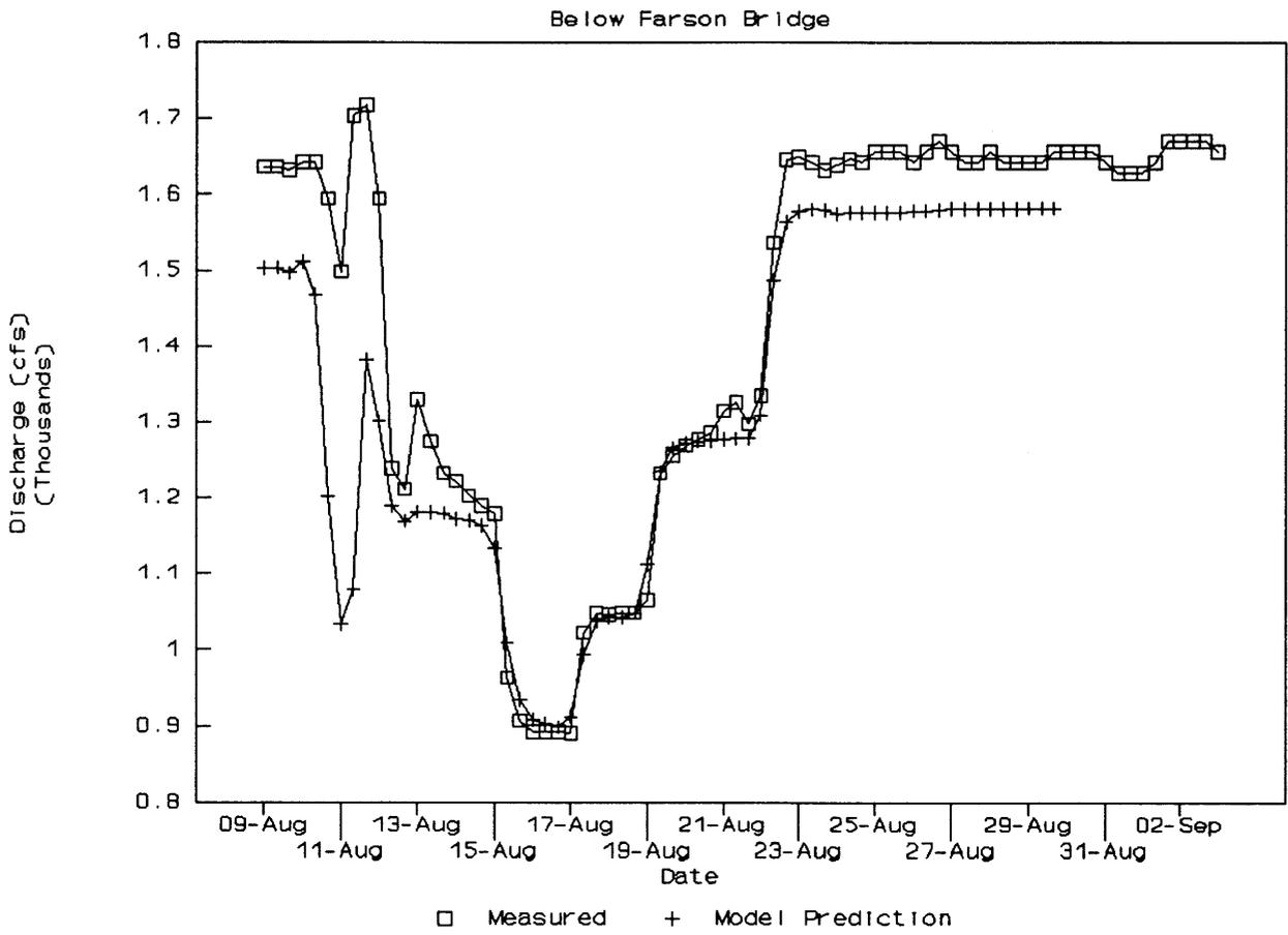
Figure 18. Green River Model Calibration of the Reach Below Farson Bridge.
