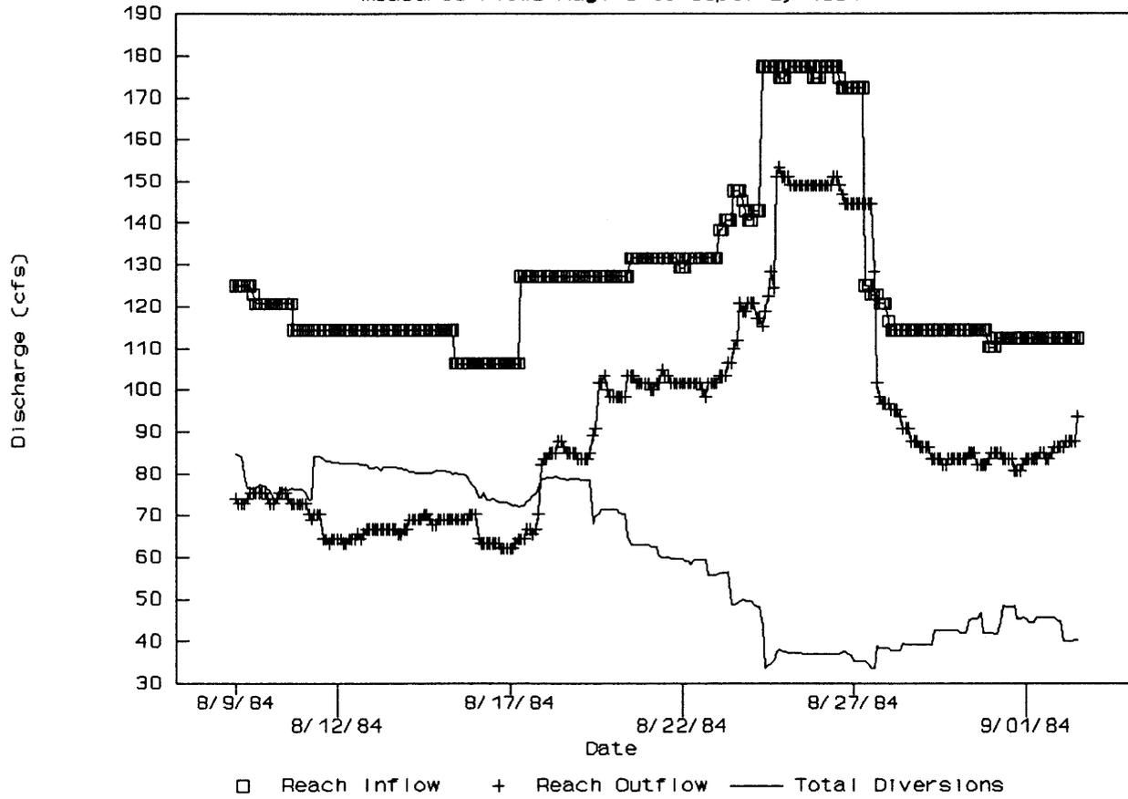
Figure 5. Piney Creek 1984 Reservoir Release, Measured Streamflow Hydrographs.
