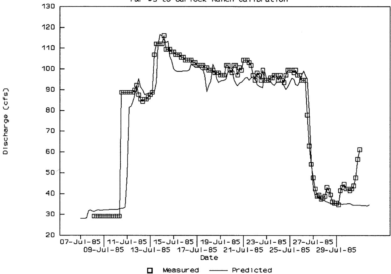
Figure 15. Clear Creek 1985 Reservoir Release, Below Pratt & Ferris Ditch No. 3 to Carlock Ranch Model Calibration.
