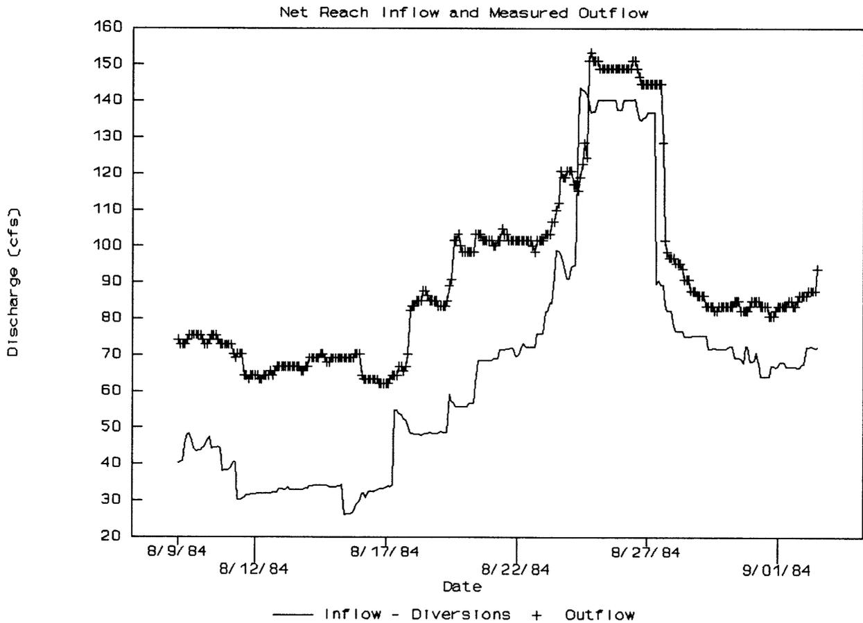
Figure 7. Piney Creek 1984 Reservoir Release, Net Reach Inflow and Measured Outflow.
