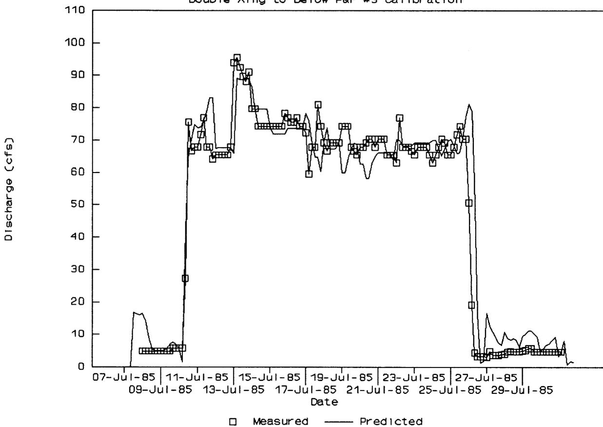
Figure 14. Clear Creek 1985 Reservoir Release, Double Crossing to Below Pratt & Ferris Ditch No. 3 Model Calibration.
