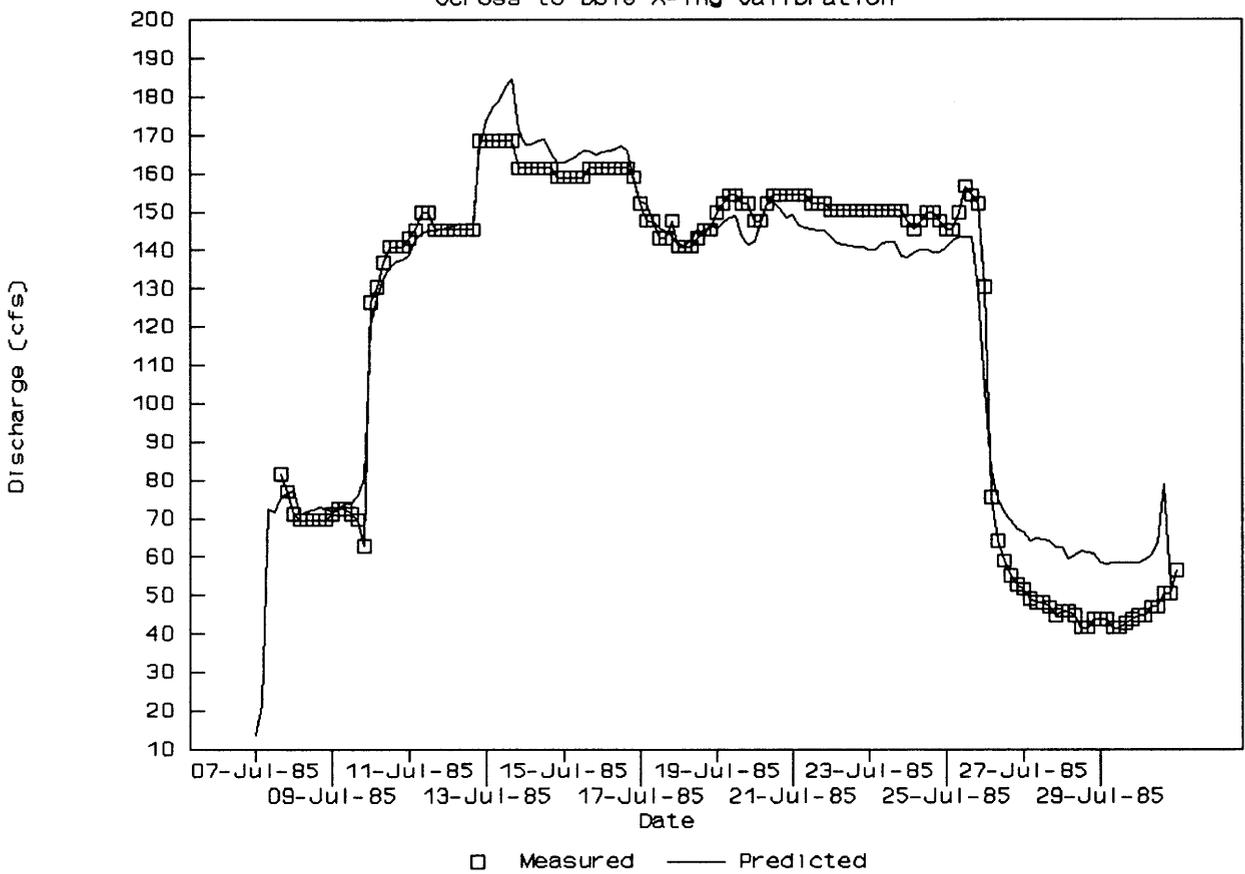
Figure 13. Clear Creek 1985 Reservoir Release, Ucross to Double Crossing Model Calibration.
