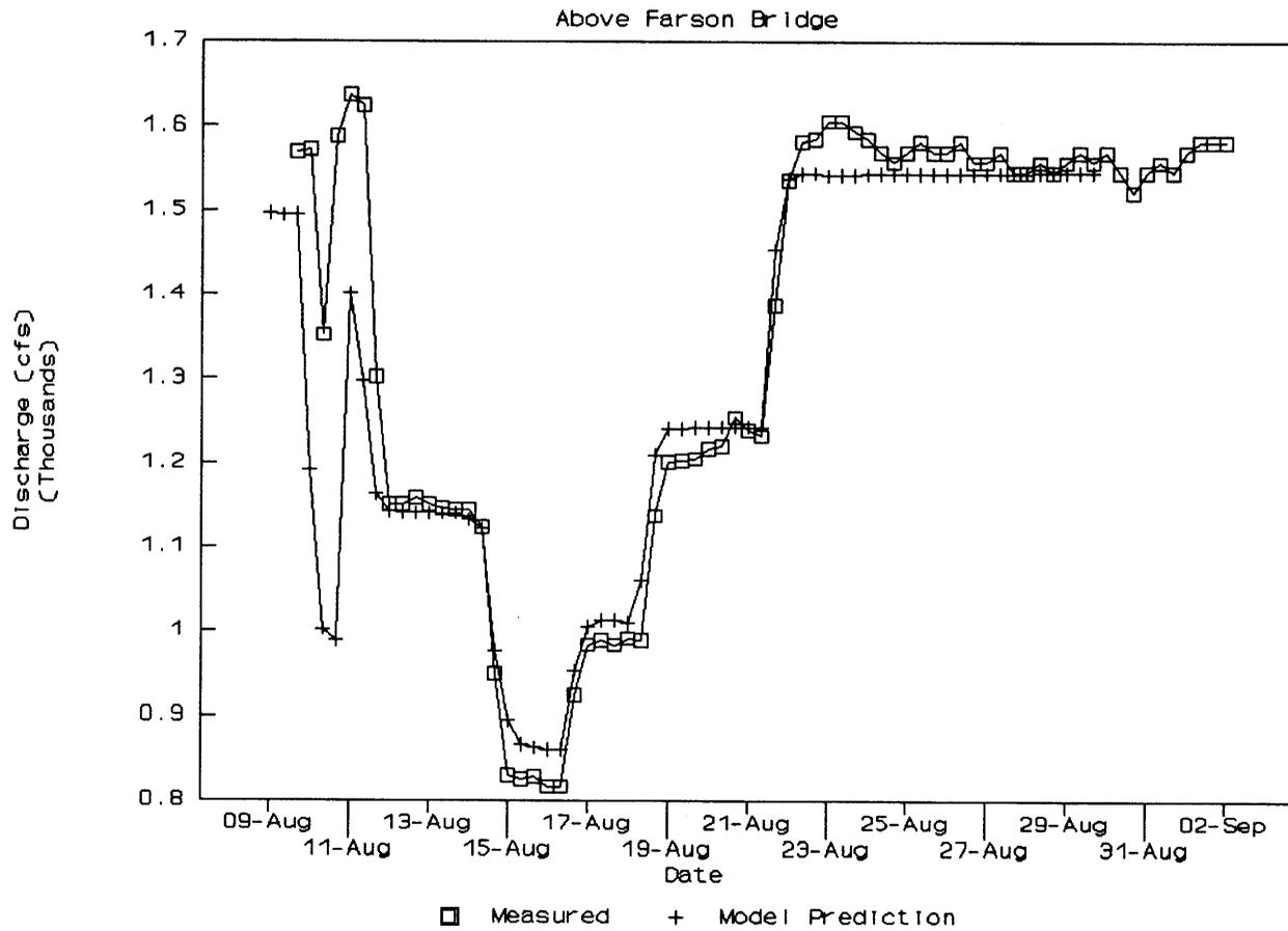
Figure 17. Green River Model Calibration of the Reach Above Farson Bridge.
