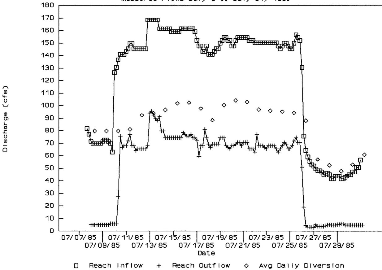
Figure 10. Clear Creek 1985 Reservoir Release, Double Crossing to Below Pratt & Ferris Ditch No. 3 Measured Streamflows.
