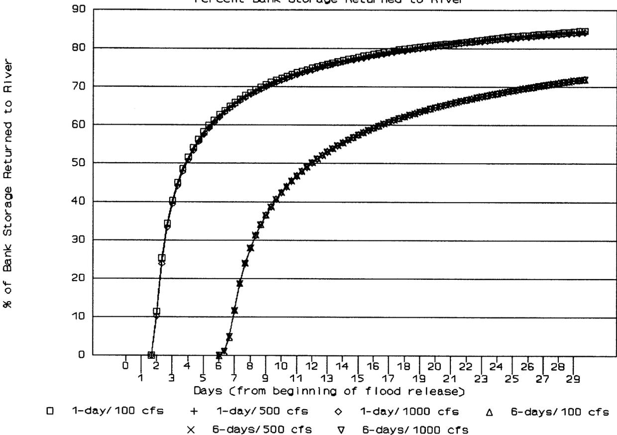
Figure 20. Green River Modeling Results of the Percent of Bank Storage Returned to the River with Varying Magnitude of Reservoir Release.
