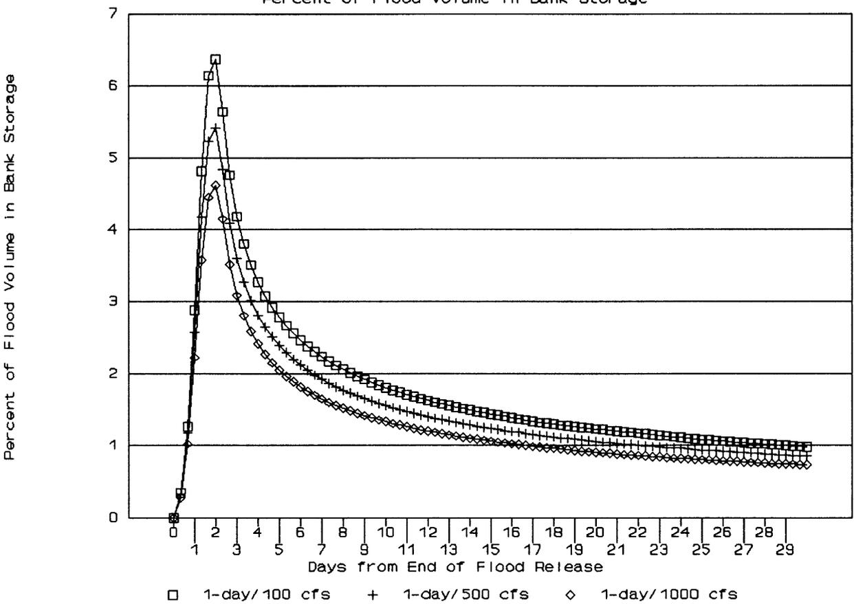
Figure 22. Green River Modeling Results, Percent of Flood Volume in Bank Storage with Varying Magnitude of Reservoir Release.
