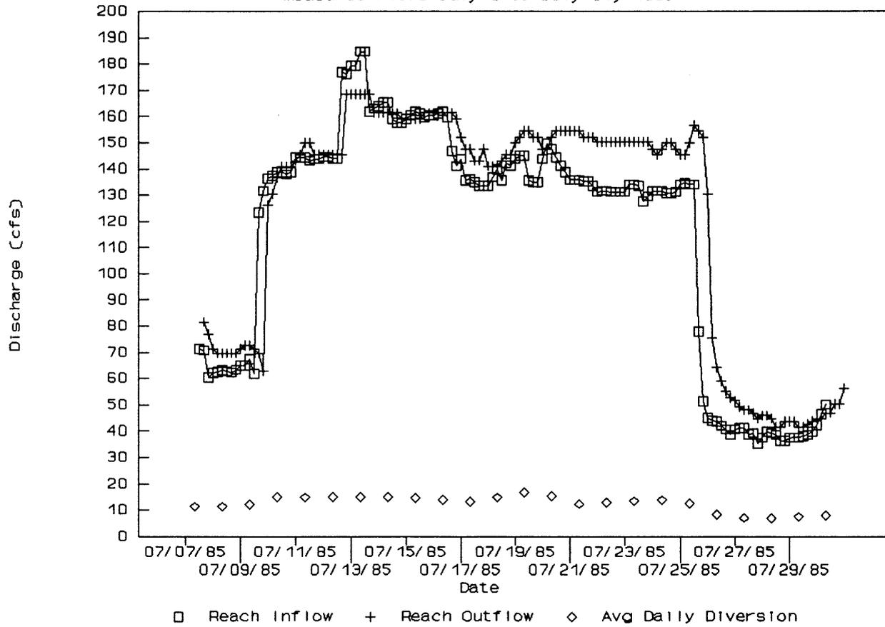
Figure 9. Clear Creek 1985 Reservoir Release, Ucross to Double Crossing Streamflows Measured.
