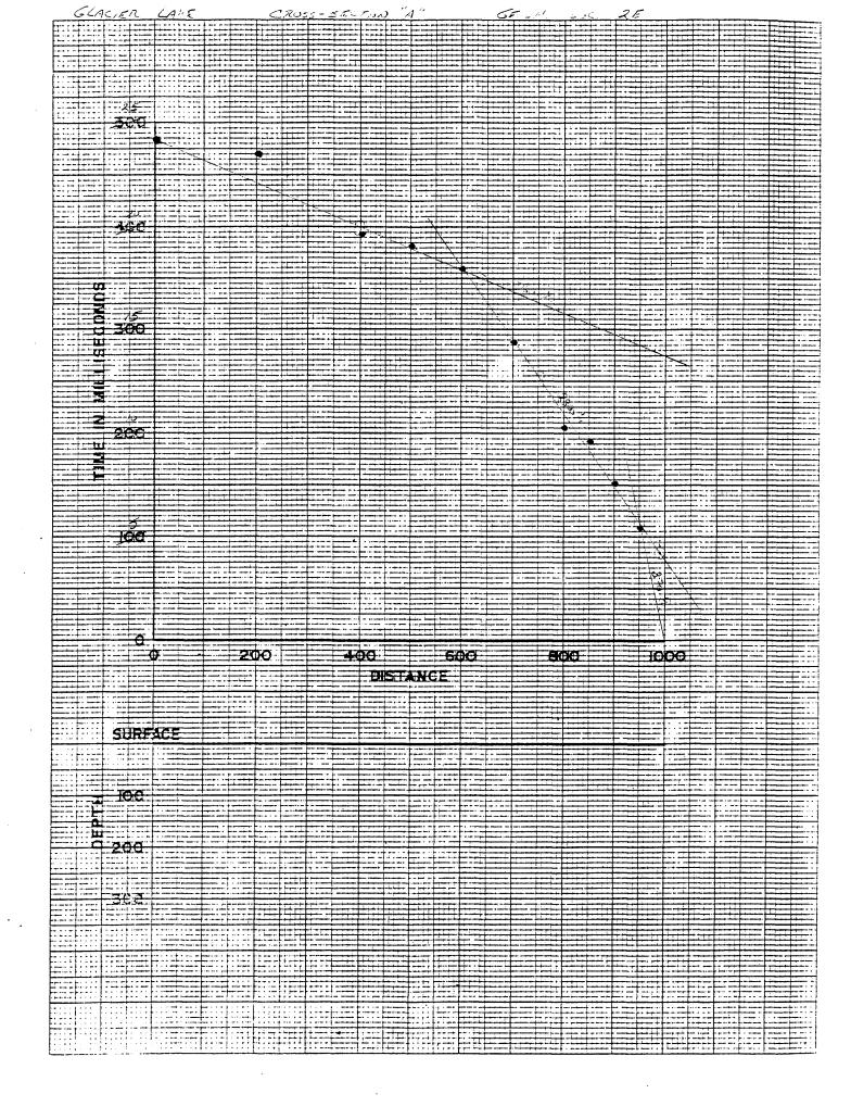
REFRACTION SURVEY "<u>B"</u> GLACIER LAKES CROSS - SECTION GEUPHONE LOCATION IW Vo = 5/4.75ms = 1050 fr/sec V = 10'/3 ms = 3333 fr/sec V2 = 221/2 ms = 11000 fr/sec Xe = 7.5 ft Tiz = 15 ms  $Z_{0} = \frac{1}{2} \sqrt{\frac{3333 - 1050}{43333}} (7.5) = 2.7 fr$  $z_{1} = \frac{1}{2} \left( .015 - 2(2.7) \frac{\sqrt{1000^{2} - 1050^{2}}}{11000(1050)} \right) \frac{11000(3333)}{\sqrt{11000^{2} - 3333^{2}}}$ = 17.3' 1111 2.7' Vo = 1050'1. V, = 3333 V. 17.3' V2 = 11000 fr/see
