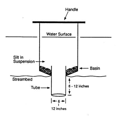
Figure 2. Drawing of a McNeil core sampler.
