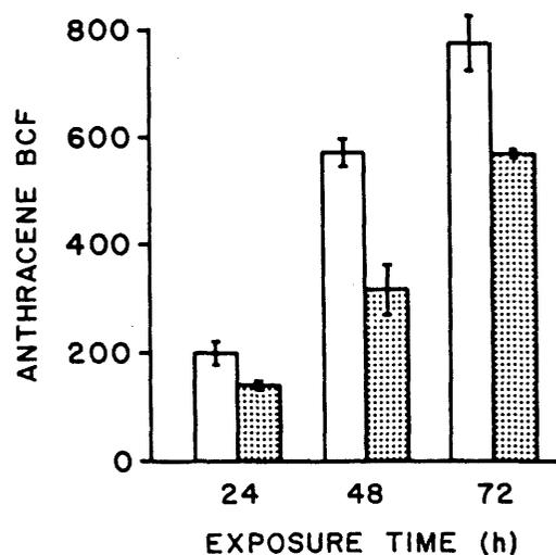
Fig. 2. Bioconcentration of [ $^{14}\text{C}$ ]anthracene in rainbow trout during the 72-h uptake period for fish exposed to either a single compound (anthracene alone, open columns) or a complex chemical mixture (anthracene in Oxy-6 retort water, stippled columns). Ranges for bioconcentration factors (BCF) in replicate aquaria are indicated for each exposure system.
