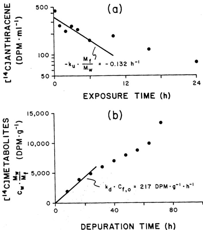
Fig. 3. Disappearance of [<sup>14</sup>C]anthracene from exposure water (a) and appearance of [<sup>14</sup>C]metabolites in depuration water (b) for one replicate of fish exposed to anthracene alone. See the text for equations.
