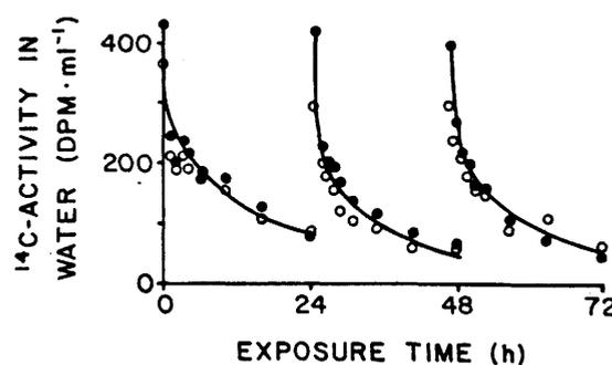
Fig. 5. Disappearance of  $[^{14}\text{C}]$ anthracene during the 72-h uptake period from exposure waters containing either a single compound (anthracene alone, filled circles) or a complex chemical mixture (anthracene in Oxy-6 retort water, open circles). Means of replicate aquaria are plotted for each exposure system.
