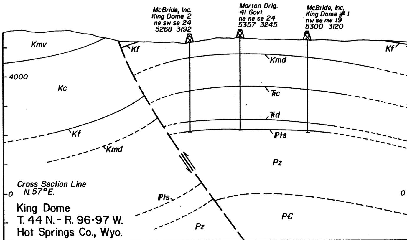
Figure 21. Structural cross section through the King Dome, Bighorn Basin, Wyoming.
