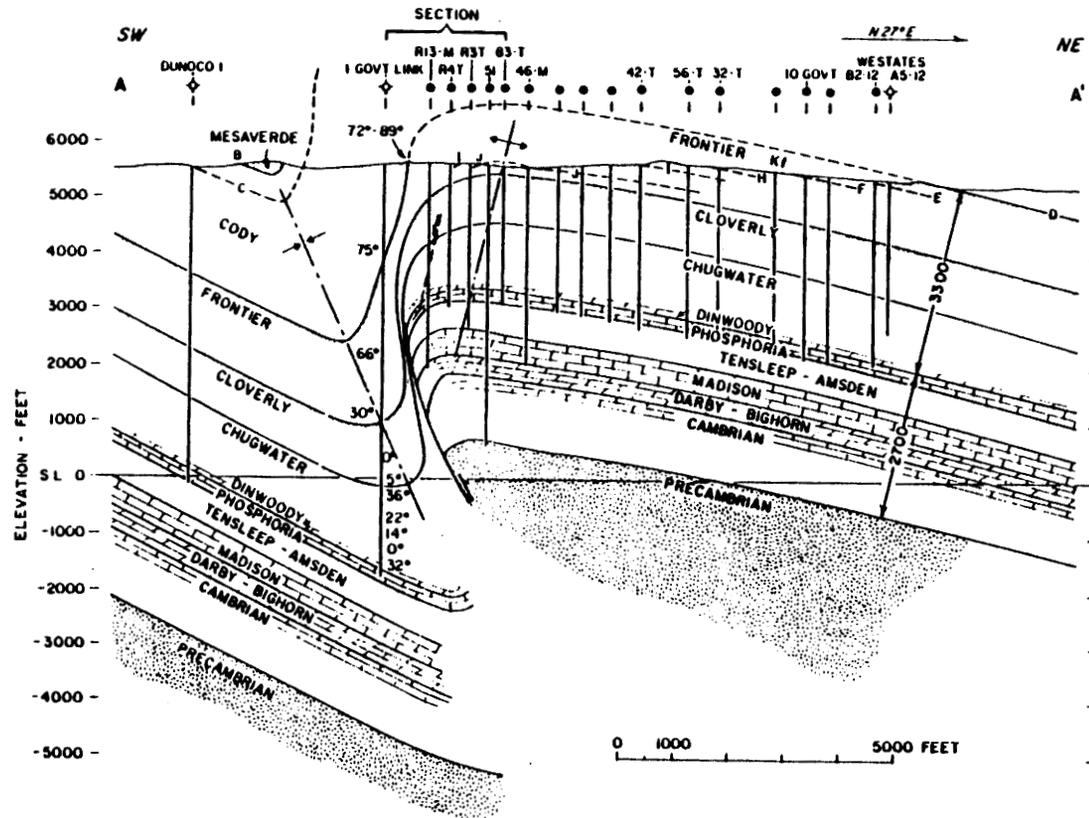
Figure 20. Structural cross section through the Hamilton Dome, Bighorn Basin, Wyoming (From Berg, 1976, Fig. 3).
