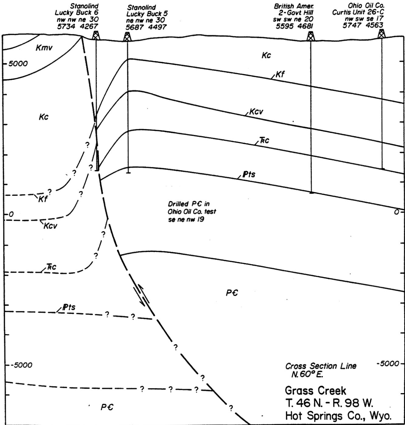
Figure 19. Structural cross section through the Grass Creek field, Bighorn Basin, Wyoming.
