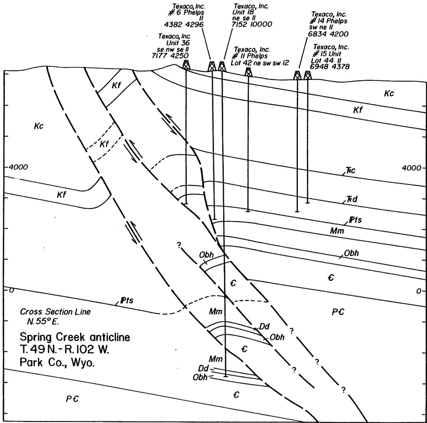
Figure 30. Structural cross section through the Spring Creek field, Bighorn Basin, Wyoming.
