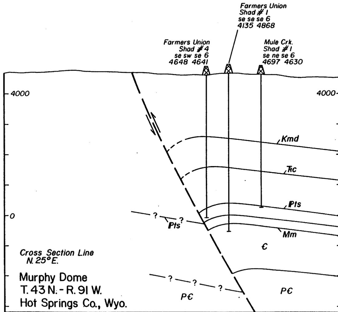
Figure 24. Structural cross section through the Murphy Dome, Bighorn Basin, Wyoming.
