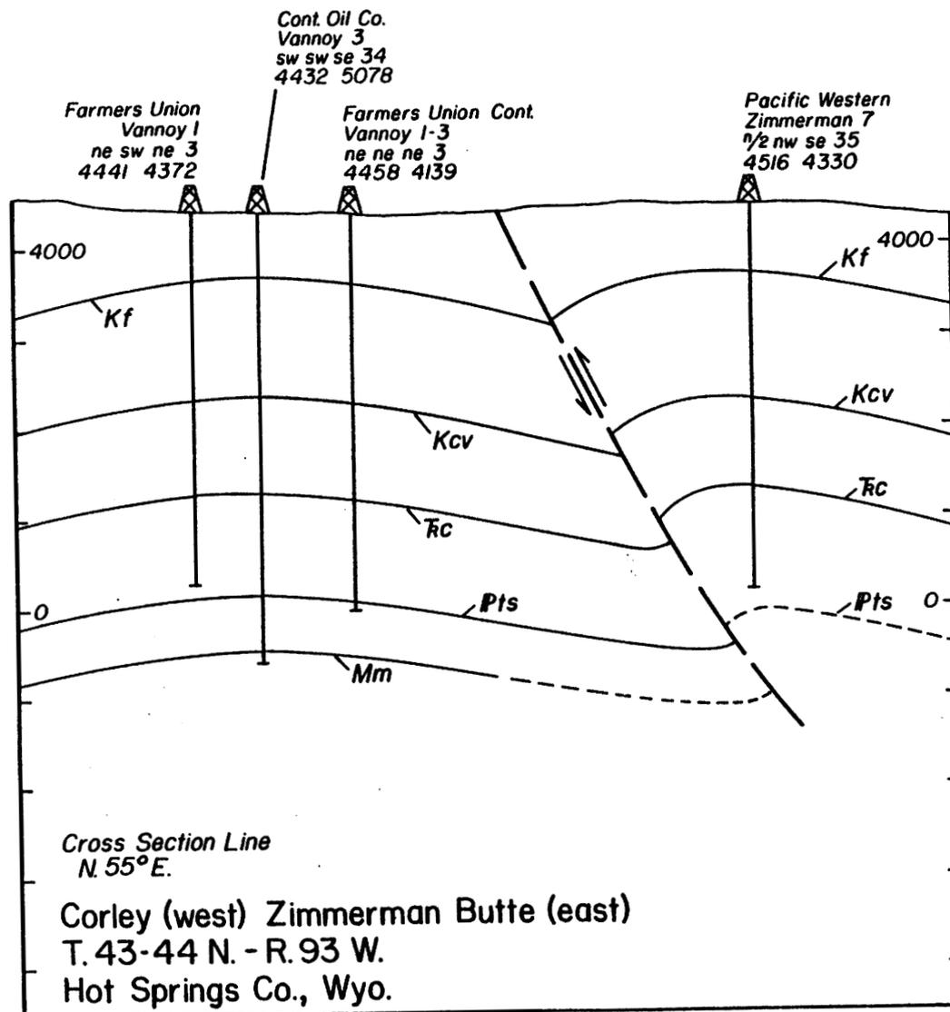
Figure 16. Structural cross section through the Corley-Zimmerman Butte folds, Bighorn Basin, Wyoming.
