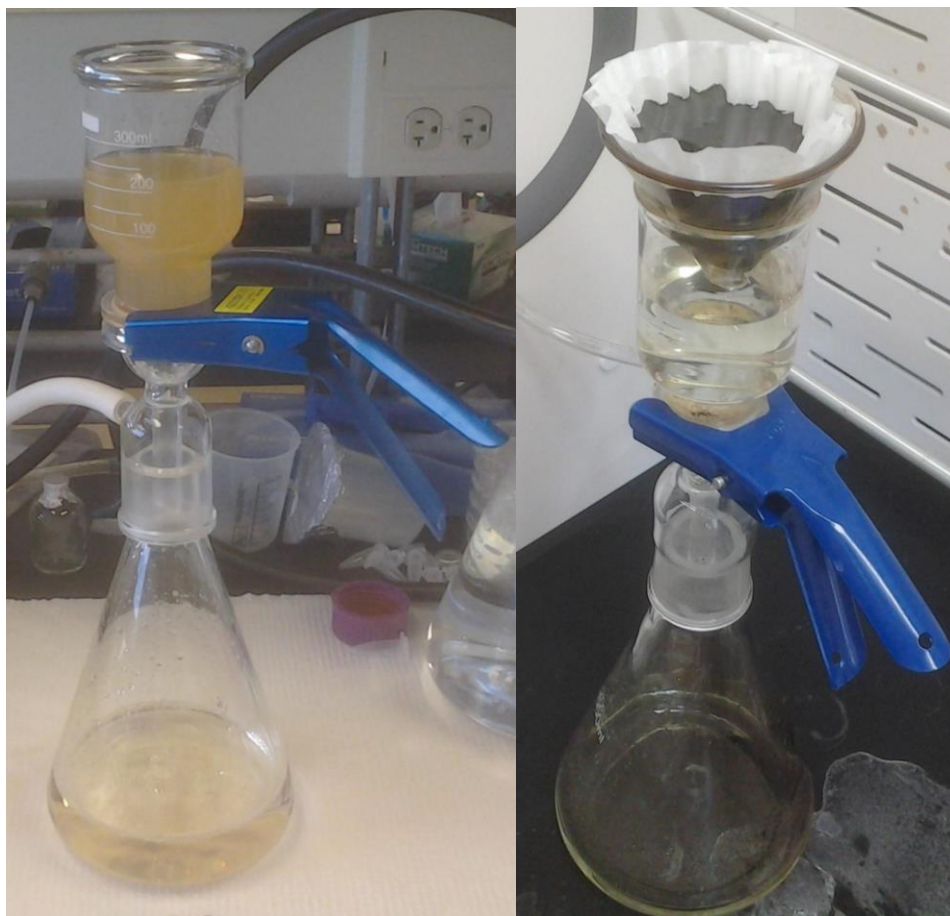
Figure 2: Two samples being filtered. The rust-colored sample on the left is typical of the PRB2 sample set and the clear sample on the right is typical of the QD sample set. When the QD sample set was filtered a coffee filter was used to separate the oil-tar from the produced water. This filter had been soaked in toluene, dried, and microwave sterilized to ensure it did not affect the microbial rRNA extracted as part of the Metagenomic methods.
