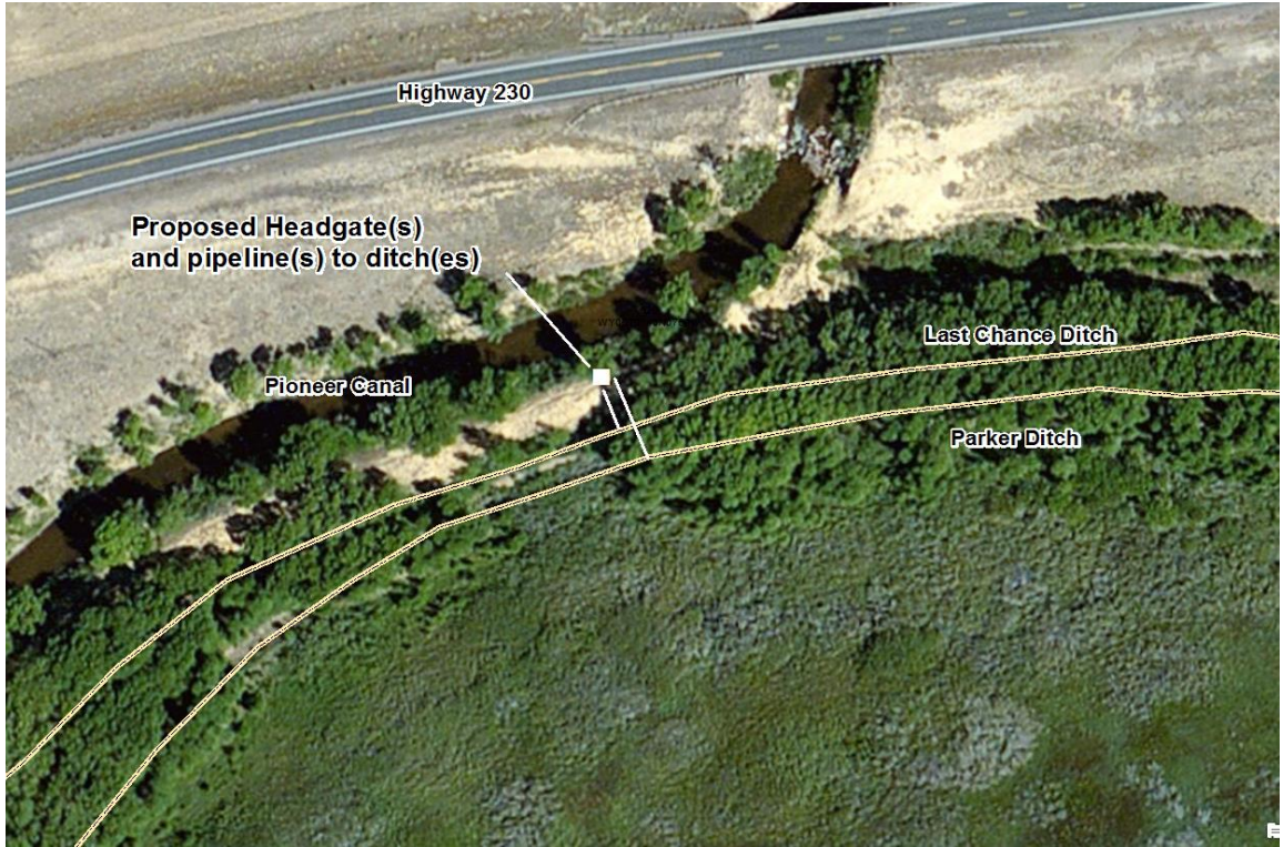
Figure 4.4-10 Proposed Headgate Relocation for Parker and/or Last Chance Ditch.
