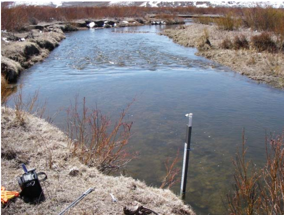
Beaver Creek (570,200E, 4,761,500N, NAD 83, UTM zone 12) example of an F-type channel with entrenchment ratio of 1.33, width/depth ratio of 31, sinuosity greater than 1.2, slope of 0.2%.
