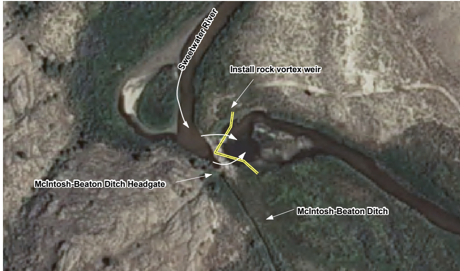
Figure 3.4 McIntosh-Beaton Ditch Rehabilitation.
