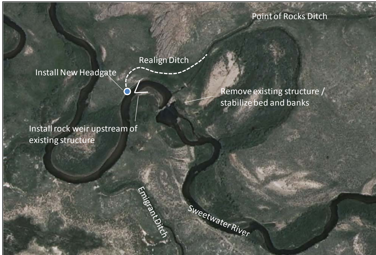
Figure 3.4 Point of Rocks Diversion Structure Conceptual Design.
