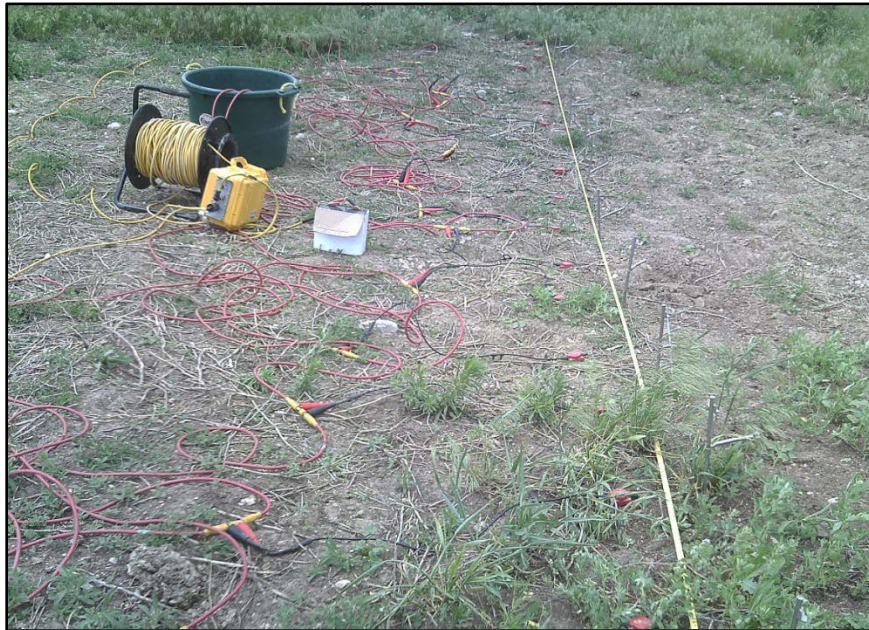
Photo shows geo-phones installed for the seismic survey.
