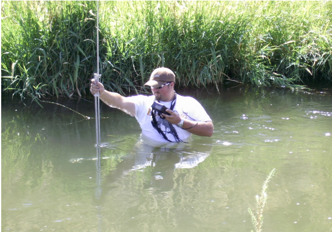
Photo 6.2.3.1: Flow measurement of canal cross section
