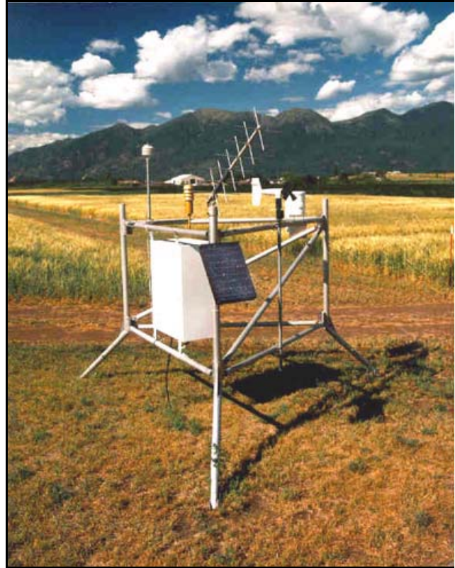
Figure 8.5 Typical AgriMet Weather Station (Photo USBR).
