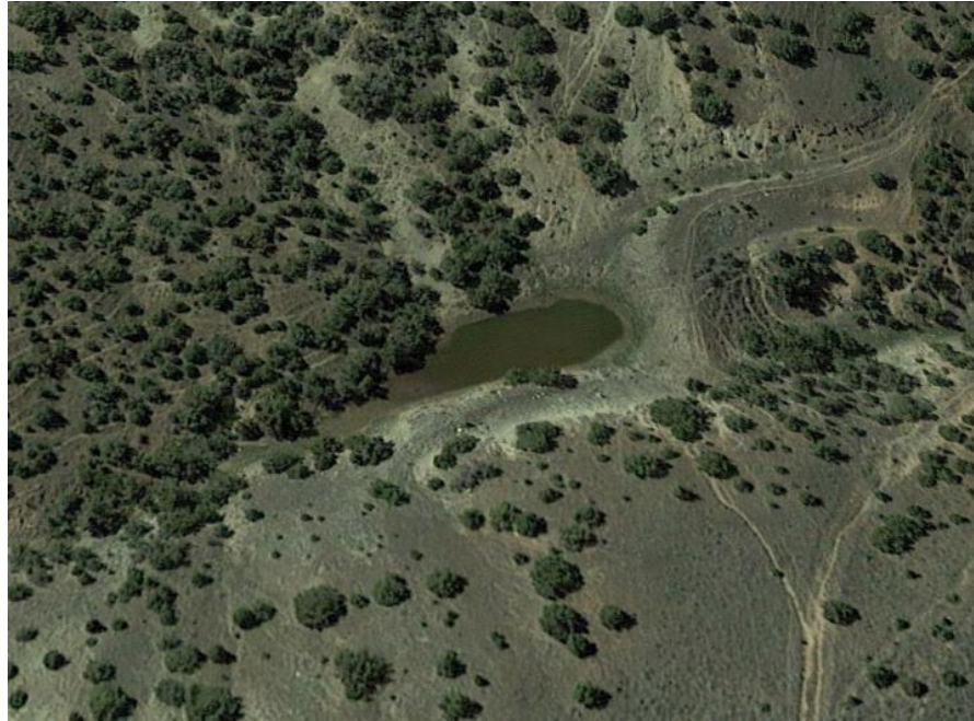
Figure 3.9.3-2a. Example of a Functional reservoir, no physical breeches or sedimentation. (Source: NAIP Imagery 2015)
