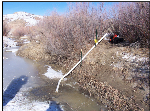
Figure 3.42 Temporary Stream Gage Installed on Cottonwood Creek
