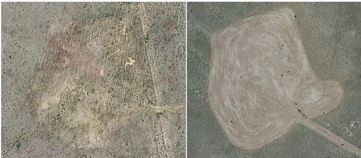
Figure 3.3-17 Example analysis of abandoned oil/gas well site. The site on the left displays vegetation cover equivalent with its surroundings, while the site on the right displays little, if any, vegetation establishment.
