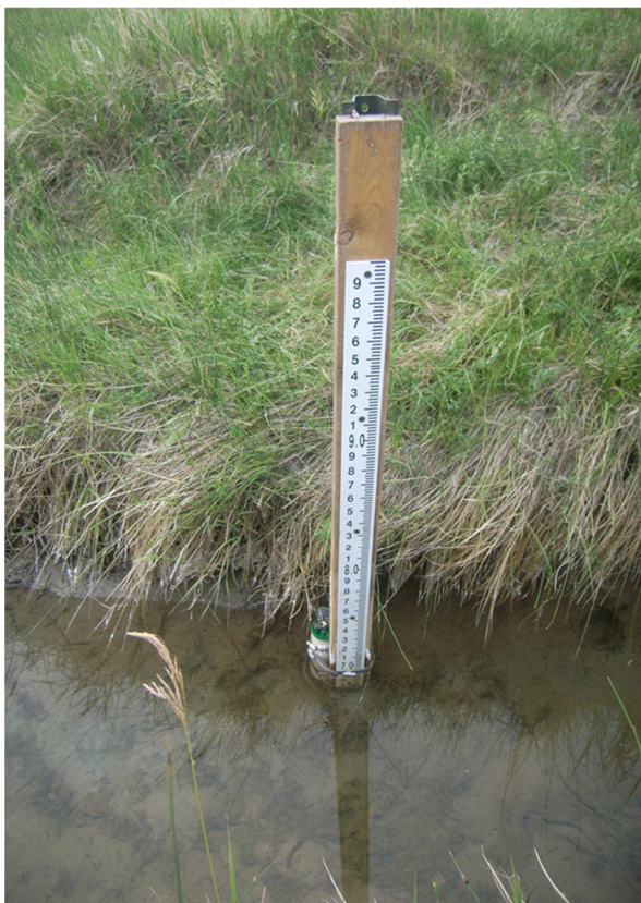
Figure 3.44. Temporary Stream Gage Installed on East Fork Bates Creek.
