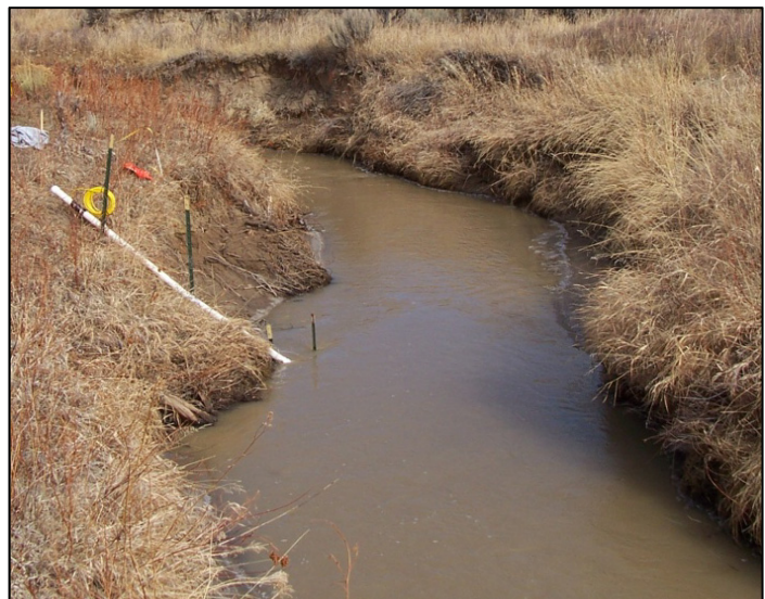
Figure 3.5-7 Temporary Stream Gage Installed in Willow Creek.
