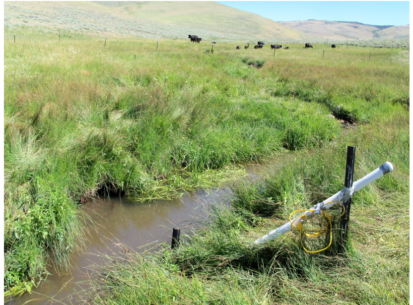
Figure 3.40 Temporary Stream Gage Installed in Antelope Creek.
