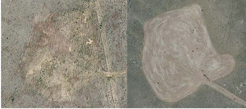
Figure 3.3-15 Example analysis of abandoned oil/gas well site. The site on the left displays vegetation cover equivalent with its surroundings, while the site on the right displays little, if any, vegetation establishment.
