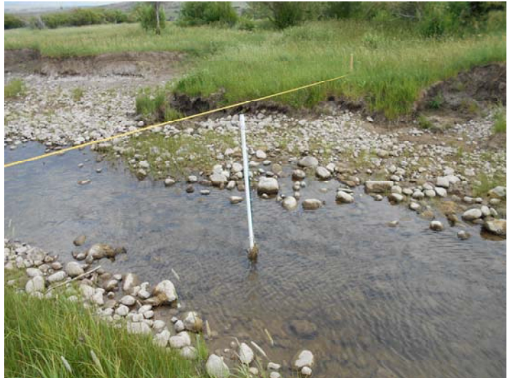
Figure 3.5-7 Temporary Stream Gage Installed in Muddy Creek.
