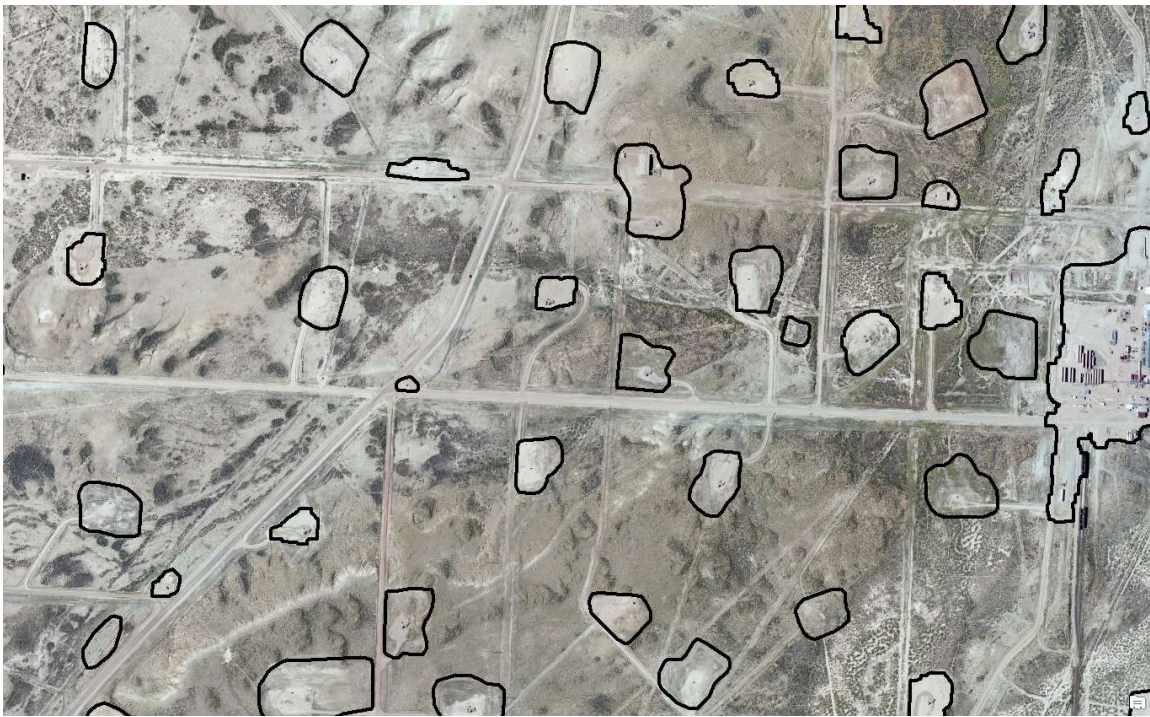
Figure 4.4-11 Example of USGS Delineation of Oil and Gas Well Pad Scars.
