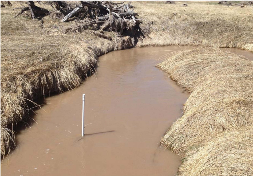
Figure 3.40. Temporary Stream Gage and Transducer Installed on Lytle Creek.
