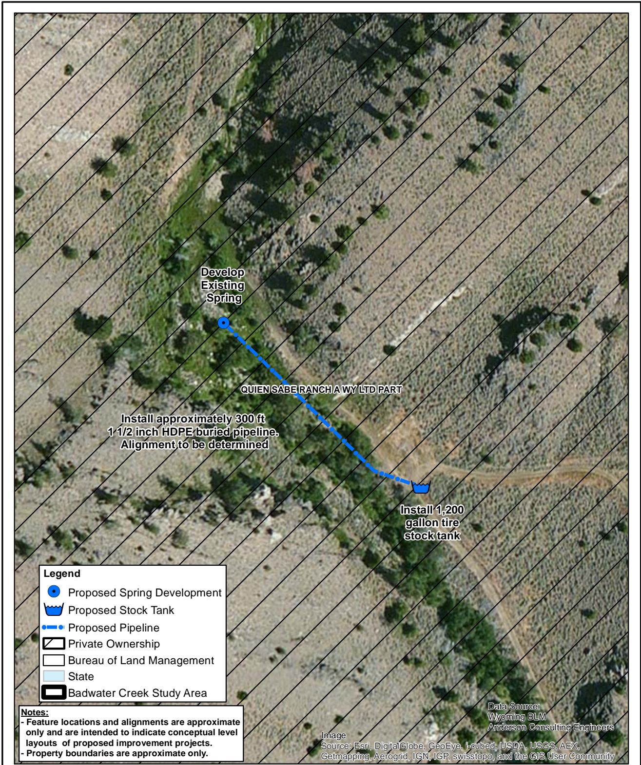
Figure 4.3-26 Conceptual Design L/W-24: Thoren Upland Water Supply Project 3
