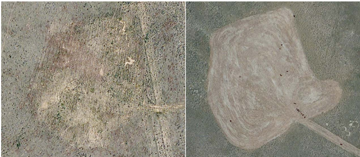
Figure 3.3-15 Example analysis of abandoned oil/gas well site. The site on the left displays vegetation cover equivalent with its surroundings, while the site on the right displays little, if any, vegetation establishment.
