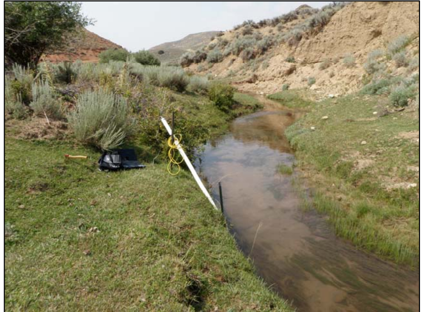
Figure 3.5-8 Temporary Stream Gage Installed in Bridger Creek.
