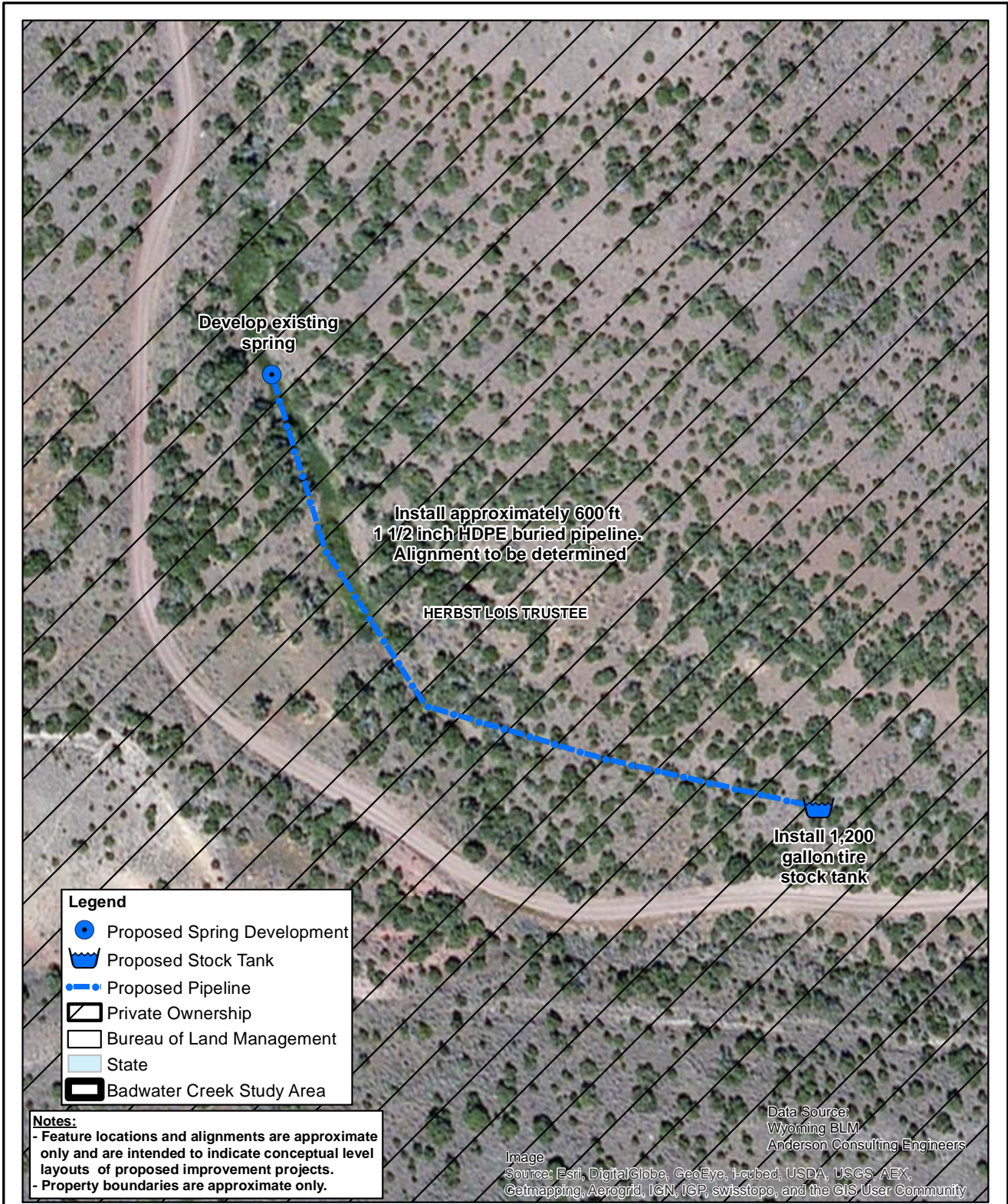
Figure 4.3-18 Conceptual Design LW-16: Cady Upland Water Supply Project 3
