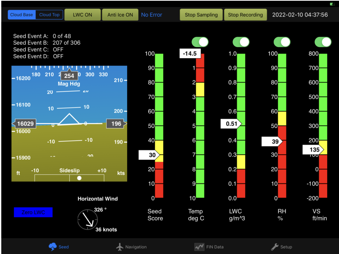
Figure 15. A screenshot of the CWIP iPad. This screen shows the primary CWIP display used by the crew in flight to monitor seeding conditions. Its display includes horizontal wind, seed score, temperature, liquid water content (LWC), relative humidity (RH), and vertical speed (VS). Seed score is a mathematical calculation based on several of these measurements. Although interesting to see, it should be noted that it is only as good as the measurement it is taking and should be interpreted with caution. For example, if the aircraft is seeding above the cloud layer using ejectable flares, the seed score is inaccurate as the instrument is in clear air and is not sampling what is being seeded below the aircraft (ejectables fall downward) and downwind. Screenshot by Captain Alex Salsbury.
