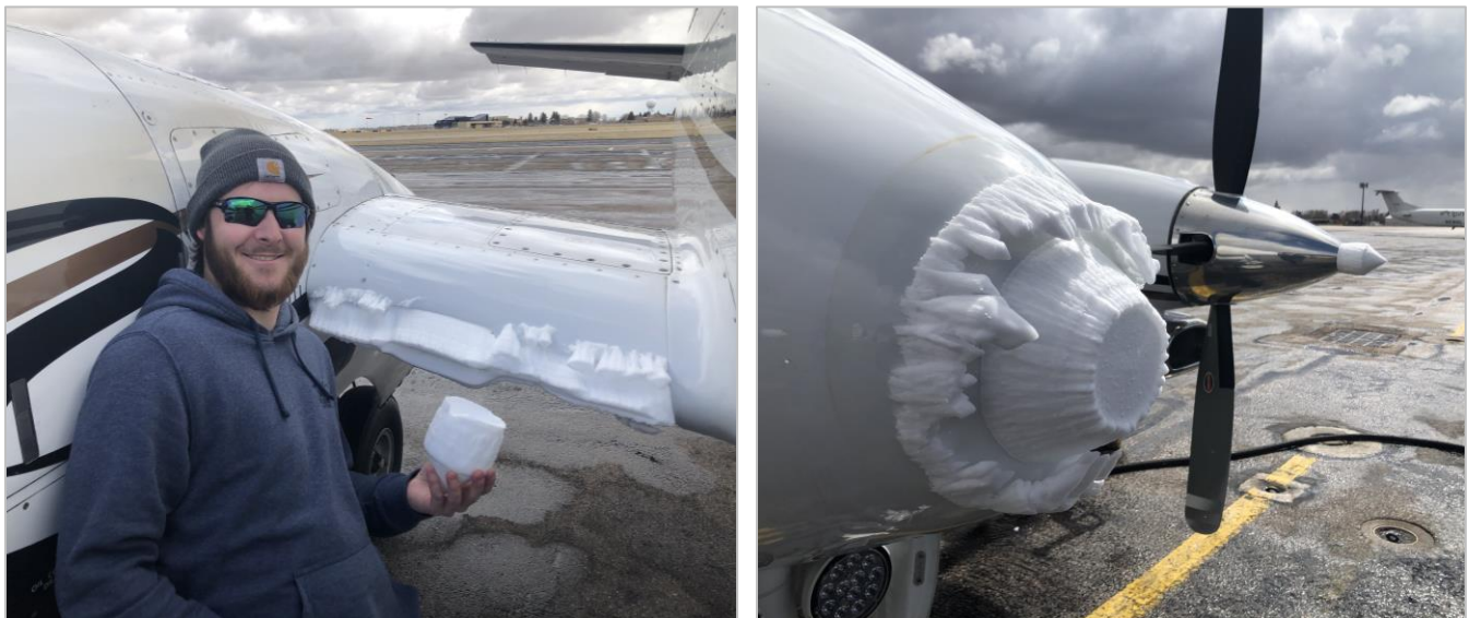
Figure 8. Images of airframe icing from 2021-2022 winter season. Left Ryan Starkey holds a piece of ice off the propeller spinner while posing next to the remains of ice buildup on the leading edge of the wing. Right – Ice buildup on the nose and propeller spinner. Both images were taken after a 5-hour mission over the Medicine Bow range on 22 March 2022. Photos by Captain Alex Sailsbury.
