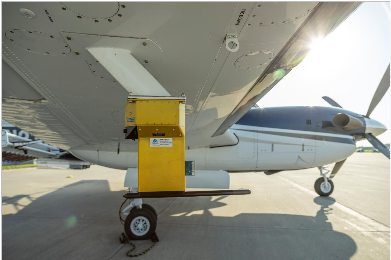
Figure 14. Cloud Water Inertial Probe (CWIP) installed under the aircraft wing. Photo by WMI.
