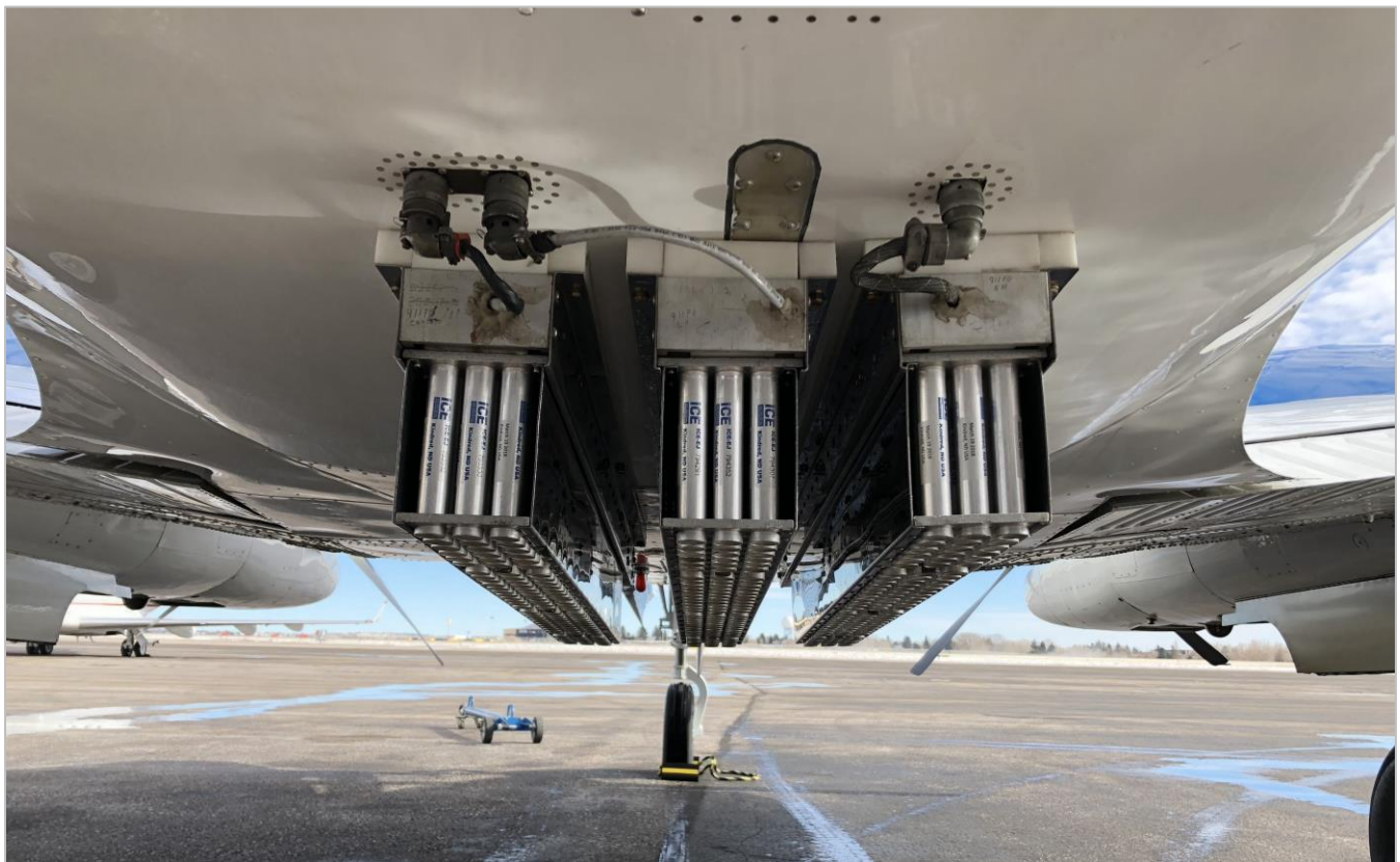
Figure 12. Ejectable flare belly racks installed on the project aircraft. Each ejectable flare yields 20g. The project aircraft was equipped as pictured with 306 ejectable flares. A total of 6,530 ICE-EJ® were expended during the 2021-2022 season. Photo by Kirk Hamilton.
