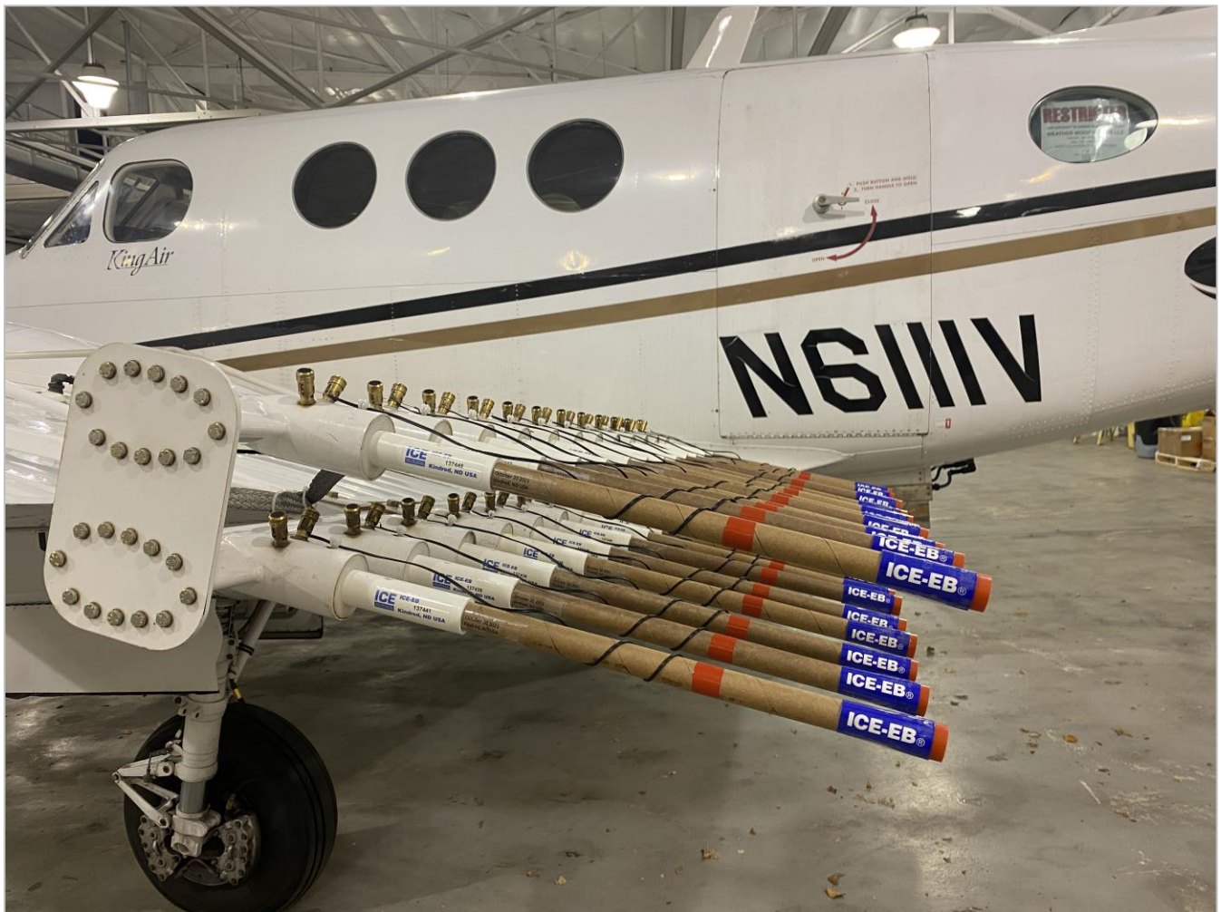
Figure 11. N6111V carried two dual burn-in-place flare racks. The flares shown are 150g ICE-EB® Ice Crystal Engineering LLC glaciogenic flares. A total of 511 ICE-EB™ flares were expended during the 2021-2022 season. Photo by Kirk Hamilton.
