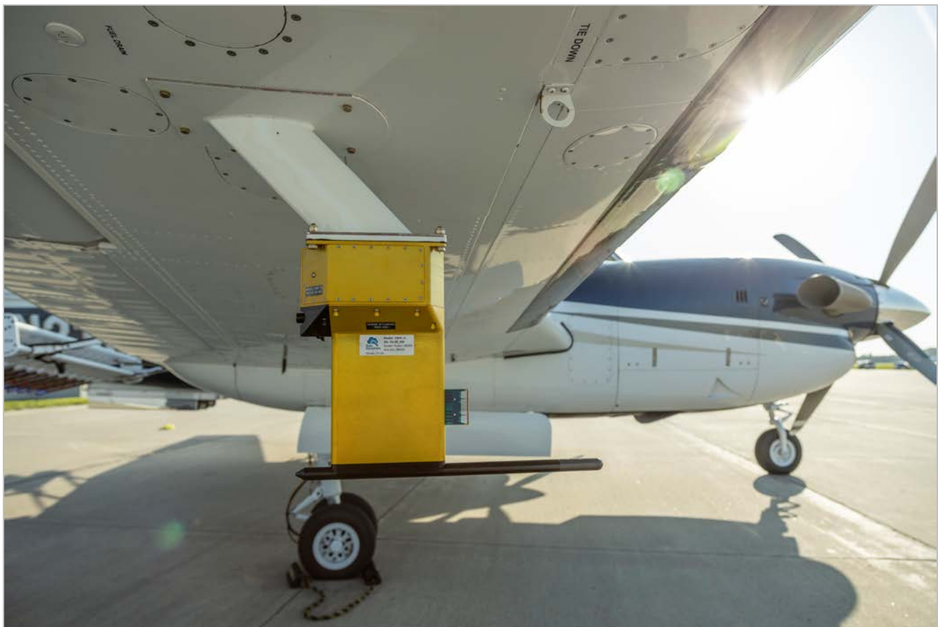
Figure 13. Cloud Water Inertial Probe (CWIP) installed under the aircraft wing. Photo by WMI.
