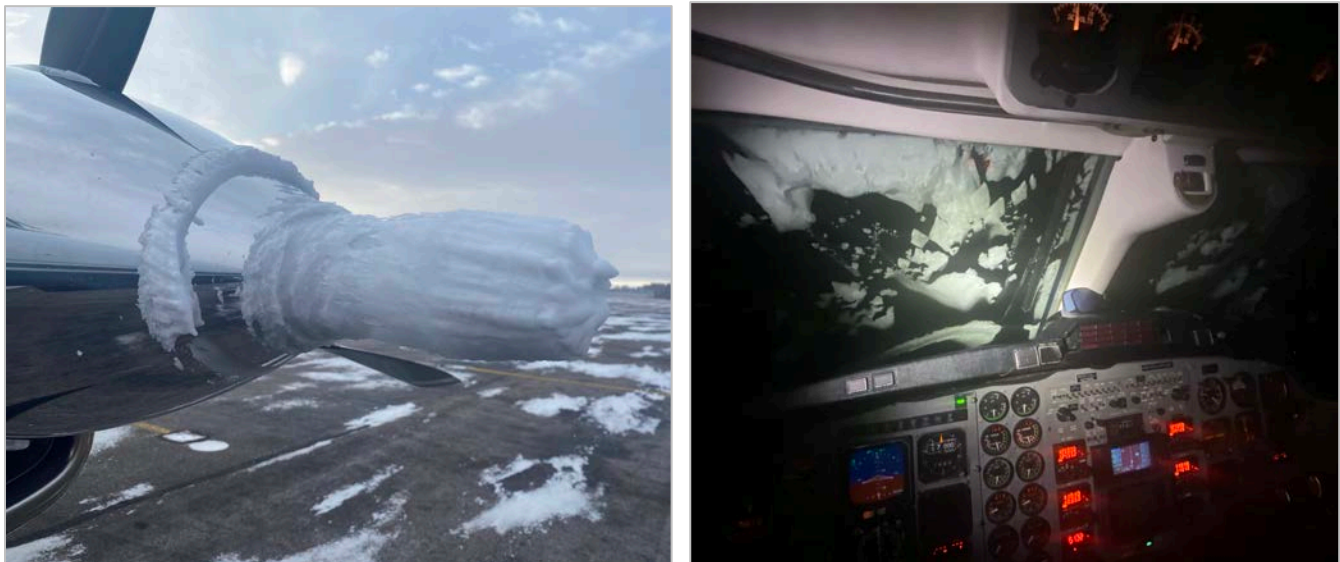
Figure 8. Images of airframe icing from 2020-2021 winter season. Left – Ice remains on the propeller spinner after the crew's first mission on 18 January 2021 for the Sierra Madre target area. The aircraft refueled and reflared after this photo was taken and departed for the Never Summer target area. Combined the aircraft flew 11 hours and 53 minutes this day. Right – Windshield icing during a night mission over the Medicine Bow target area on 9 February 2021. Photos by Kirk Hamilton.
