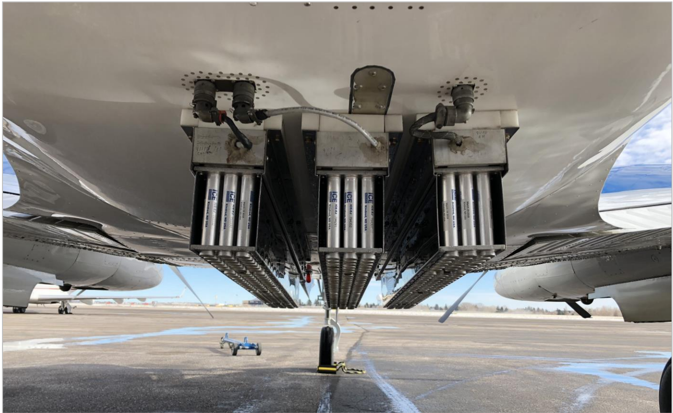
Figure 14. Ejectable flare belly racks installed on the project aircraft. Each ejectable flare yields 20g. All three project aircraft were equipped as pictured with 306 ejectable flares. A total of 4,912 ICE-EJ™ were expended during the 2019-2020 season. Photo by Kirk Hamilton.
