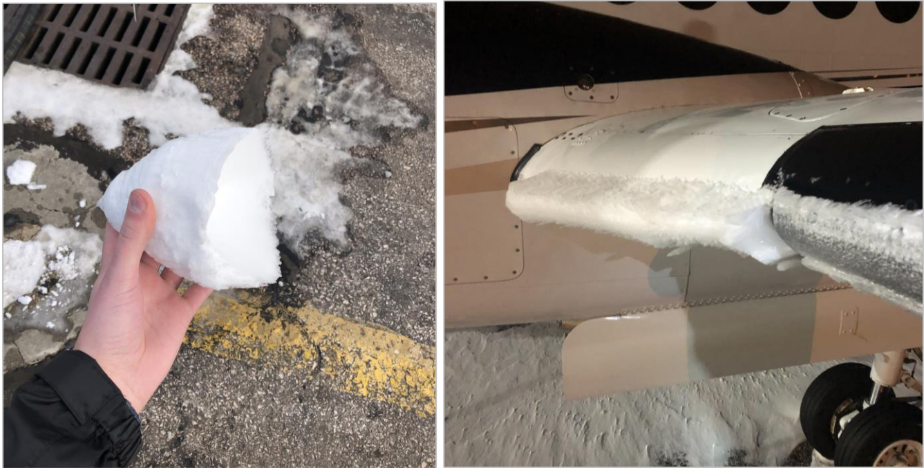
Figure 9. Images of in-flight airframe icing during WY missions on 1 Jan 2020 (left) and 9 December 2019 (right). Left – WMI copilot Tyler Couch holds a piece of ice off the propeller spinner after a mission for the Medicine Bow target area. Photo by Tyler Couch. Right – Airframe icing after a mission on 8 December 2019 over the Laramie and Medicine Bow target area. Visible is the difference between the ice accumulations on the wing area without de-icing boots vs. the area with boots (black, far right of image) where the ice was intermittently shed throughout the flight. Photo by Kirk Hamilton.
