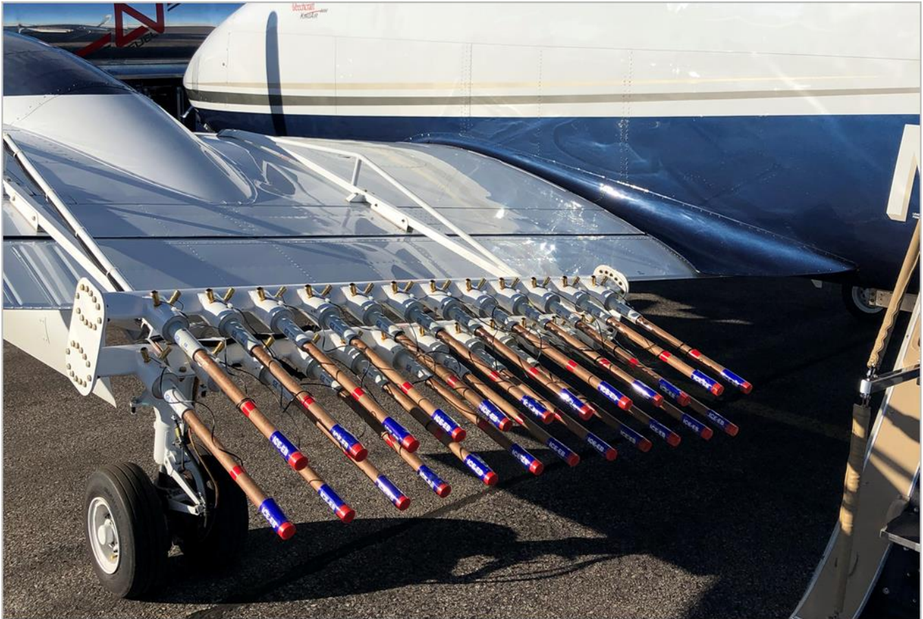
Figure 13. N23MN carried two dual burn-in-place flare racks. The flares shown are 150g ICE-EB™ Ice Crystal Engineering LLC glaciogenic flares. A total of 413 ICE-EB™ flares were expended during the 2019-2020 season. Photo by Tyler Couch.
