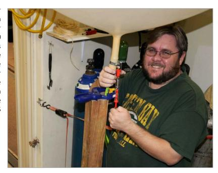
Figure 11. Meteorologist Dan Gilbert checks a weather balloon to verify that it has enough lift, prior to tying it off and attaching the meteorological instrument package. Sensors measured temperature, humidity, pressure, and position. Minute-to-minute changes in position were used to calculate wind speed and direction. (WMI photograph by Bruce Boe.)
