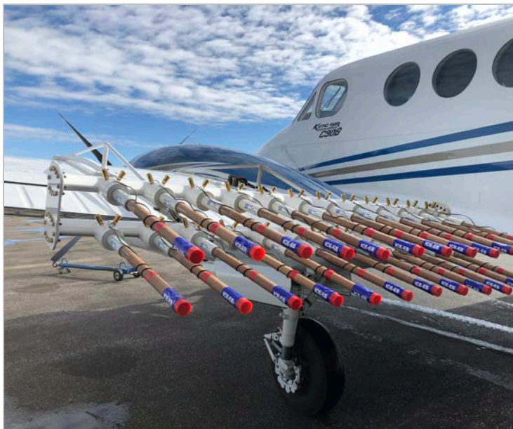
Figure 10. N127ZW aircraft carried two dual burn-in-place flare racks. The flares shown are 150g ICE-EB™ Ice Crystal Engineering LLC glaciogenic flares. Photo by Kirk Hamilton.
