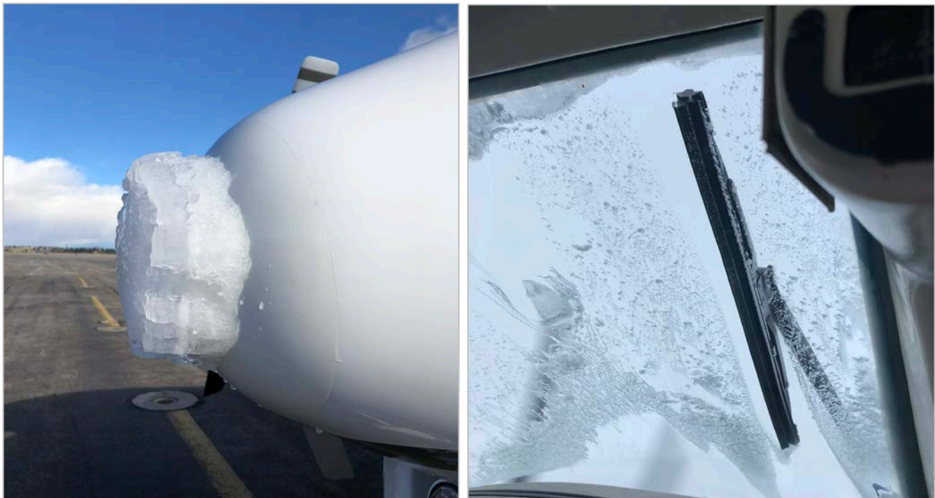
Figure 7. Images of in-flight airframe icing during WY-CO missions on February 3, 2019 (left) and November 28, 2018 (right). Left – The aircraft nose shown with icing that remained intact upon descend in Cheyenne, WY after a 5.05 hour mission for the Never Summer Mountain Range. Photo by Kirk Hamilton. Right – WMI copilot Jacob Berg captures N127ZW's windshield during a mission over the Medicine Bow Mountain Range on November 28, 2018. A total of 9.25 flight hours were flown and 13,150 grams of seeding material was dispensed during this event on the 28 th .
