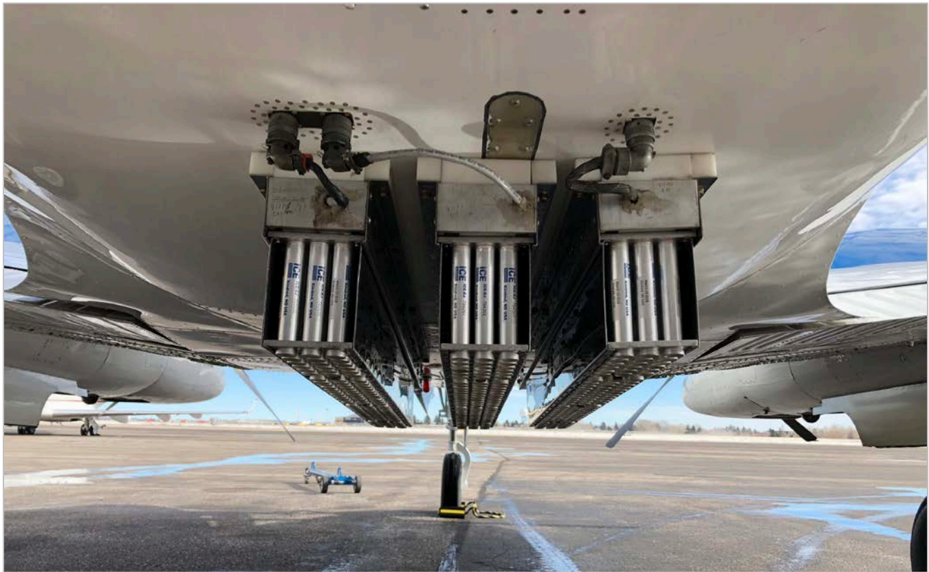
Figure 11. Ejectable flare belly racks installed on the project aircraft. Each ejectable flare yields 20g. All three project aircraft were equipped as pictured with 306 ejectable flares. Photo by Kirk Hamilton.
