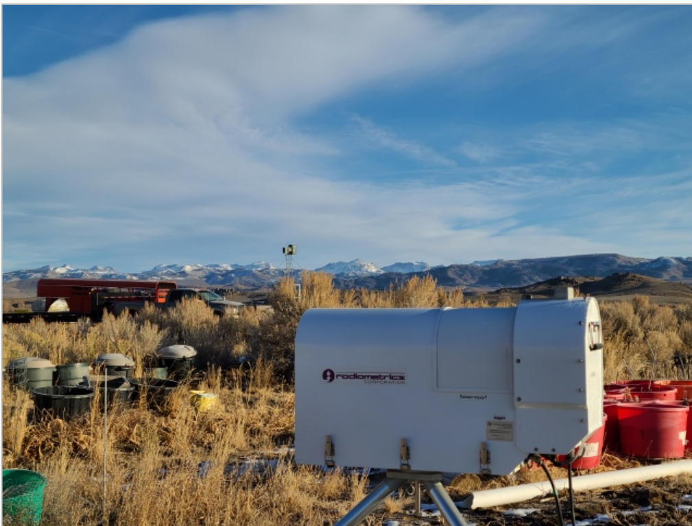
Figure 12. The radiometer is shown here, at the East Fork generator site near Boulder, WY. The instrument observes in the direction perpendicular to its axis, so as aligned here, it is configured to take measurements over the Wind River Range in the distance. The East Fork ice nucleus generator can be seen in the background, left. Photo by WMI Meteorologist Adam Brainard on 28 November 2020.
