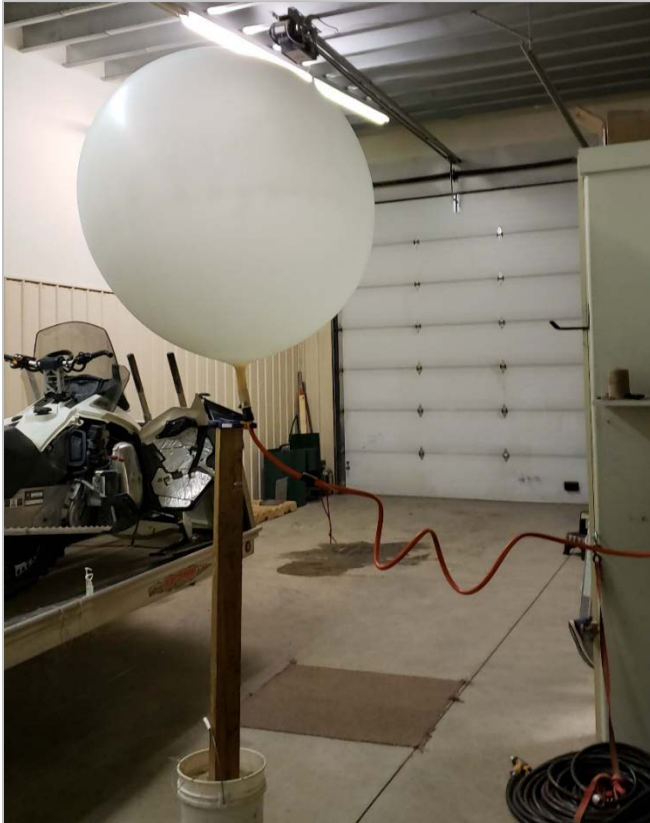
Figure 13. The weather balloon is filled, and its sonde prepared at the WMI Pinedale shop in anticipation of seedable conditions. Photo by WMI Meteorologist Jeff Ceratto on 22 December 2020.
