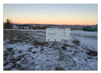
Figure 10. The radiometer sited near Cora, WY. The instrument does not transmit, but passively measures the atmospheric liquid water and water vapor. (WMI photograph by Daniel Gilbert) <u>Atmospheric Soundings</u>. The atmospheric soundings (weather balloons/rawinsondes) were discussed in Section 2.5. Data from the soundings were immediately shared with the NWS and WRDS.
