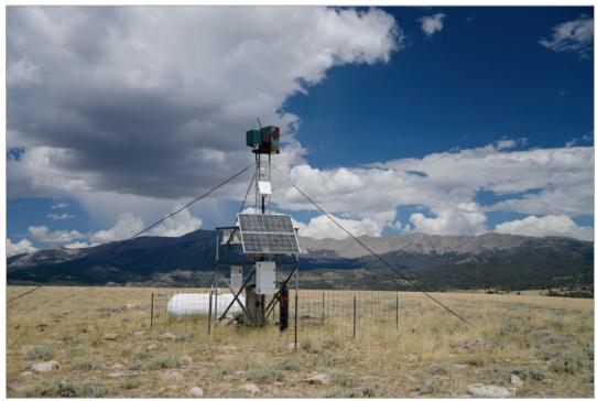
Figure 1. The ice nucleus generator sited at White Acorn Ranch on the southwest flank of the Wind River Range (WMI photograph). For the locations of all the generators, see Figure 4.
