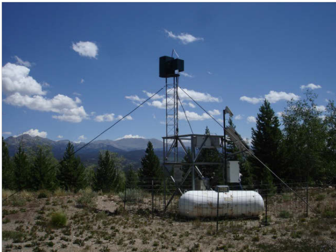
Figure 1. The ice nucleus generator sited at Big Sandy Opening on the southwest flank of the Wind River Range (WMI photograph). For the locations of all the generators, see Figure 4.
