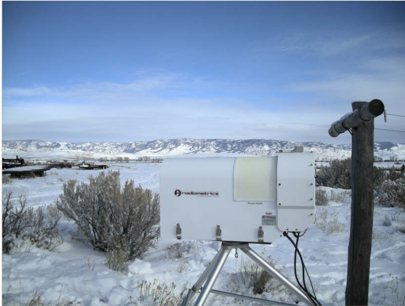
Figure 10. The radiometer sited near Boulder, WY. The instrument does not transmit, but passively measures the atmospheric liquid water and water vapor. (NCAR photograph by Daniel Breed.)
